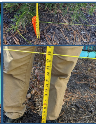
Clear photos of ponding depth and freeboard
