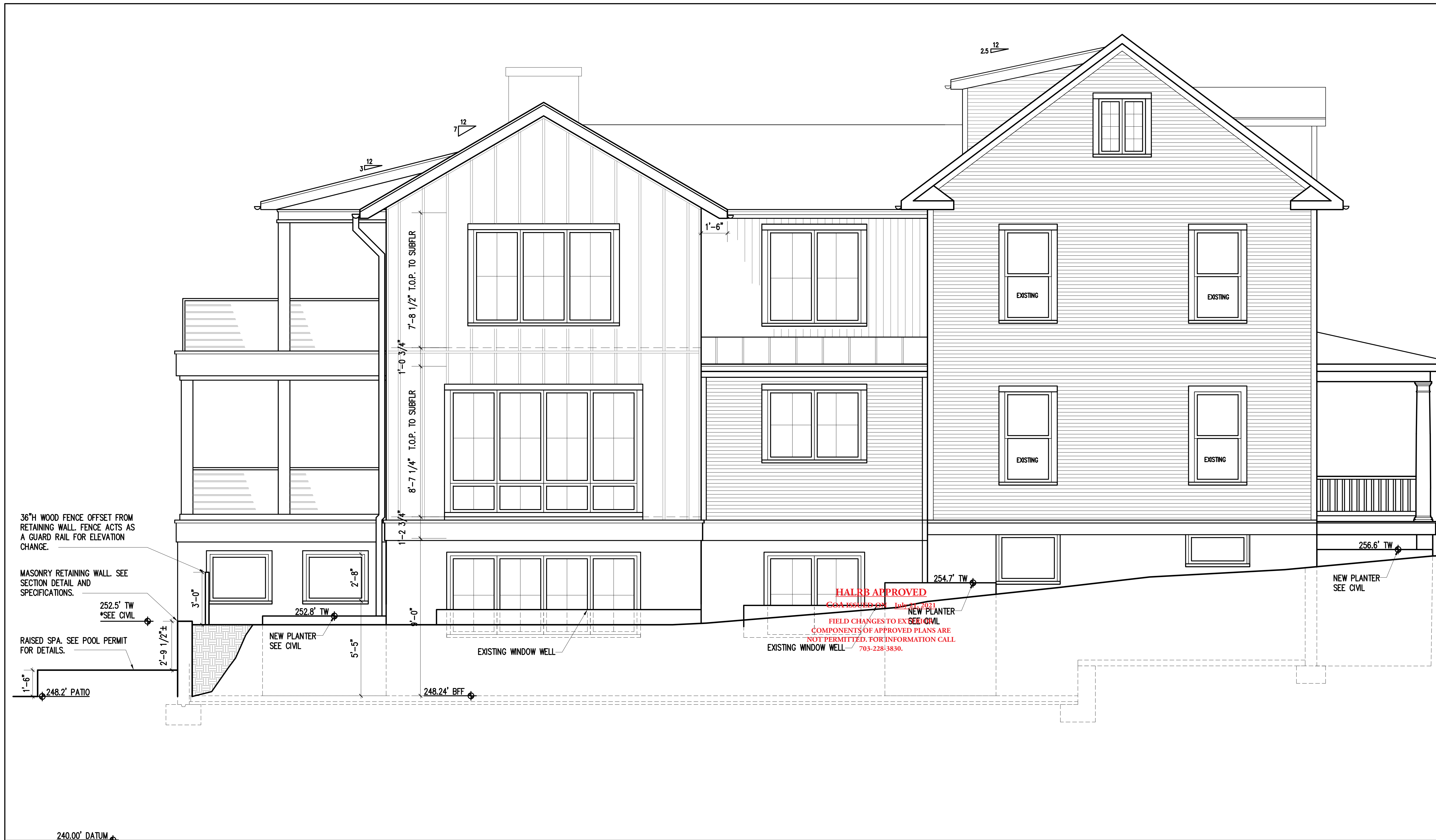
1 MAIN HOUSE EXISTING SOUTH SIDE ELEVATION Scale: 3/8" = 1'-0"
