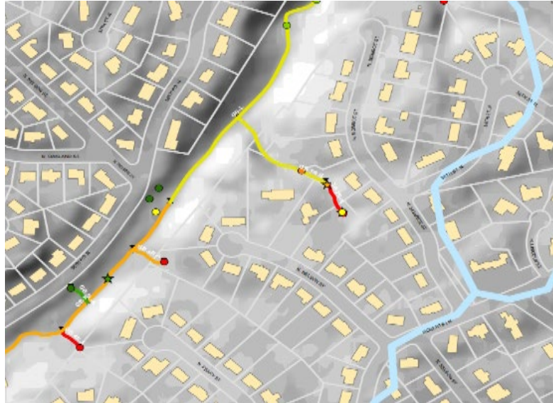
A segment of the 2011 Stream Assessment map, with colors indicating severity of erosion.
