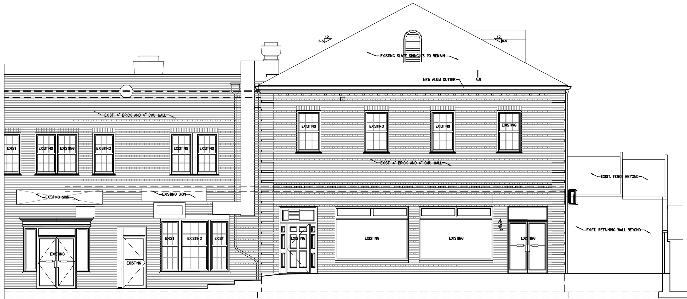
REAR ELEVATION - EXIISTING 1/8"=1'-0"
