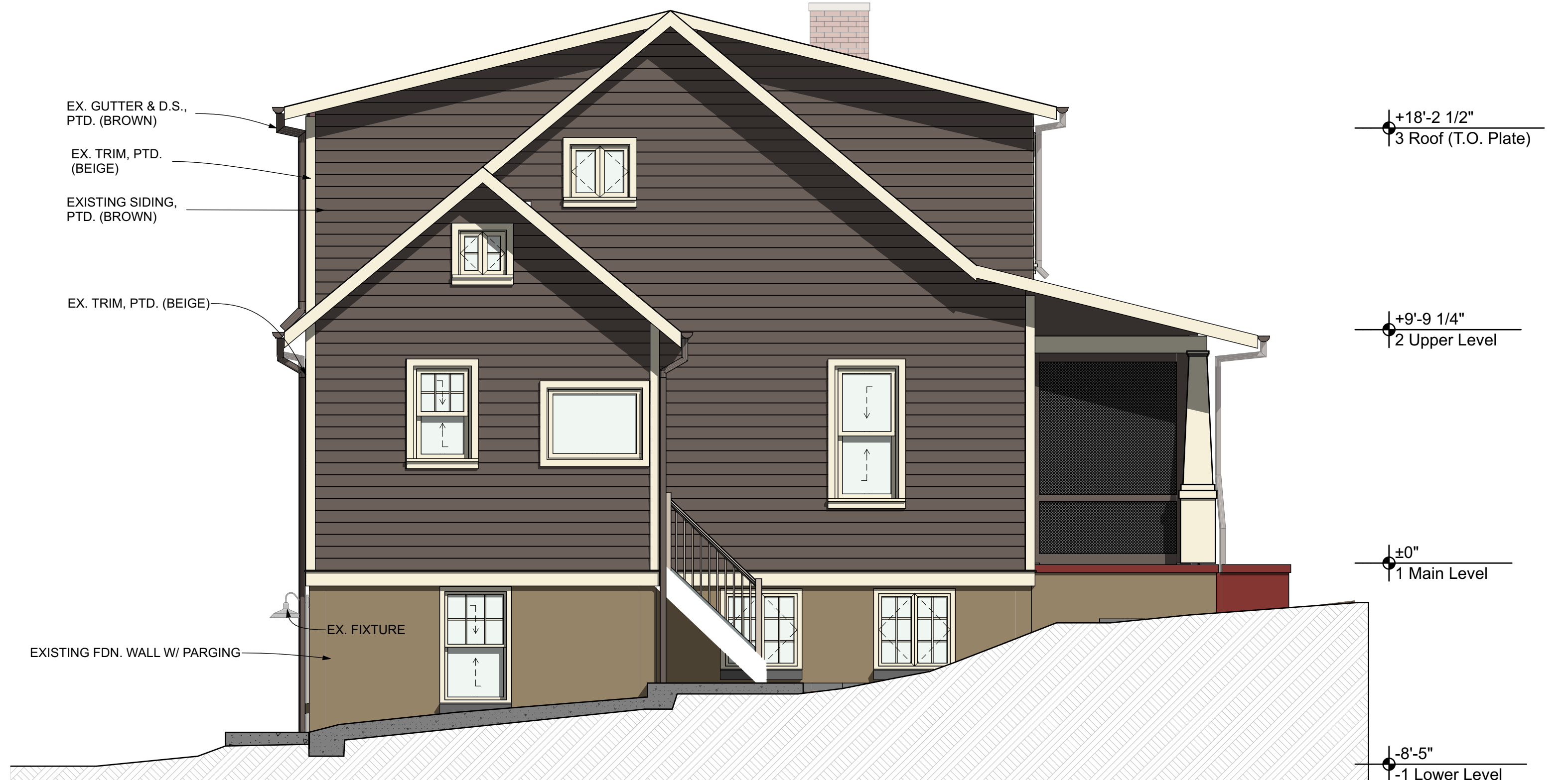
4 West Elevation - EXISTING A008 SCALE: 1/4" = 1'-0"
