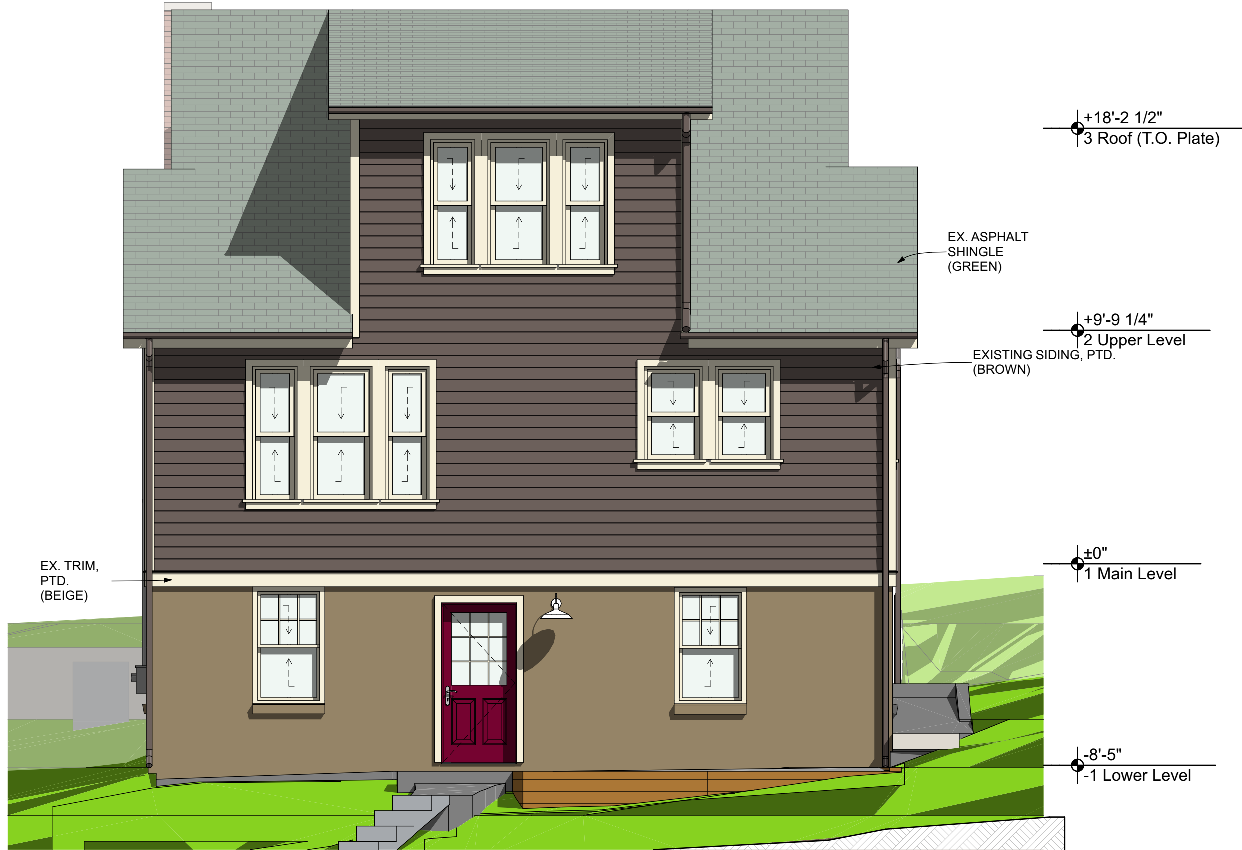
3 North Elevation - EXISTING A008 SCALE: 1/4" = 1'-0"
