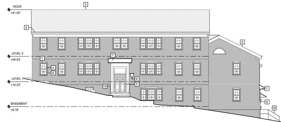
1 BLDG 26 - ELEVATION C 1/8" = 1'-0" ASE: 109.5'
