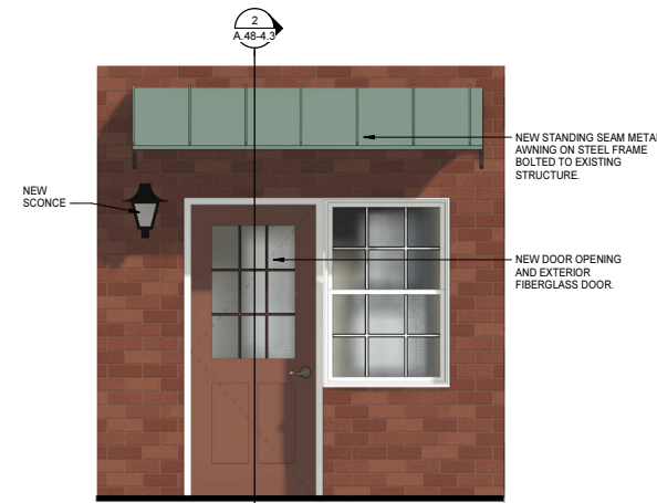
3 BLDG 48 - ENLARGED ELEVATION - ACCESSIBLE ENTRANCE 1 1/2" = 1'-0"
