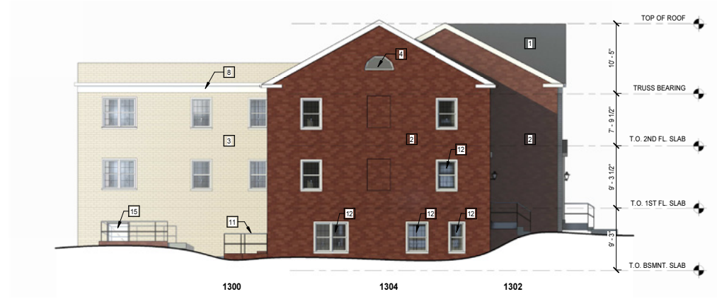
1 BUILDING 15 SOUTH ELEVATION 1/8" = 1'-0"
