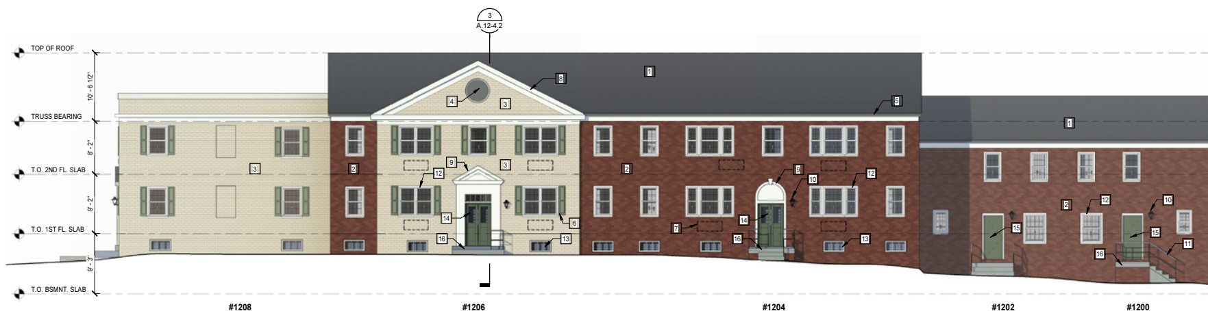
2 BUILDING 12 EAST ELEVATION 1/8" = 1'-0"
