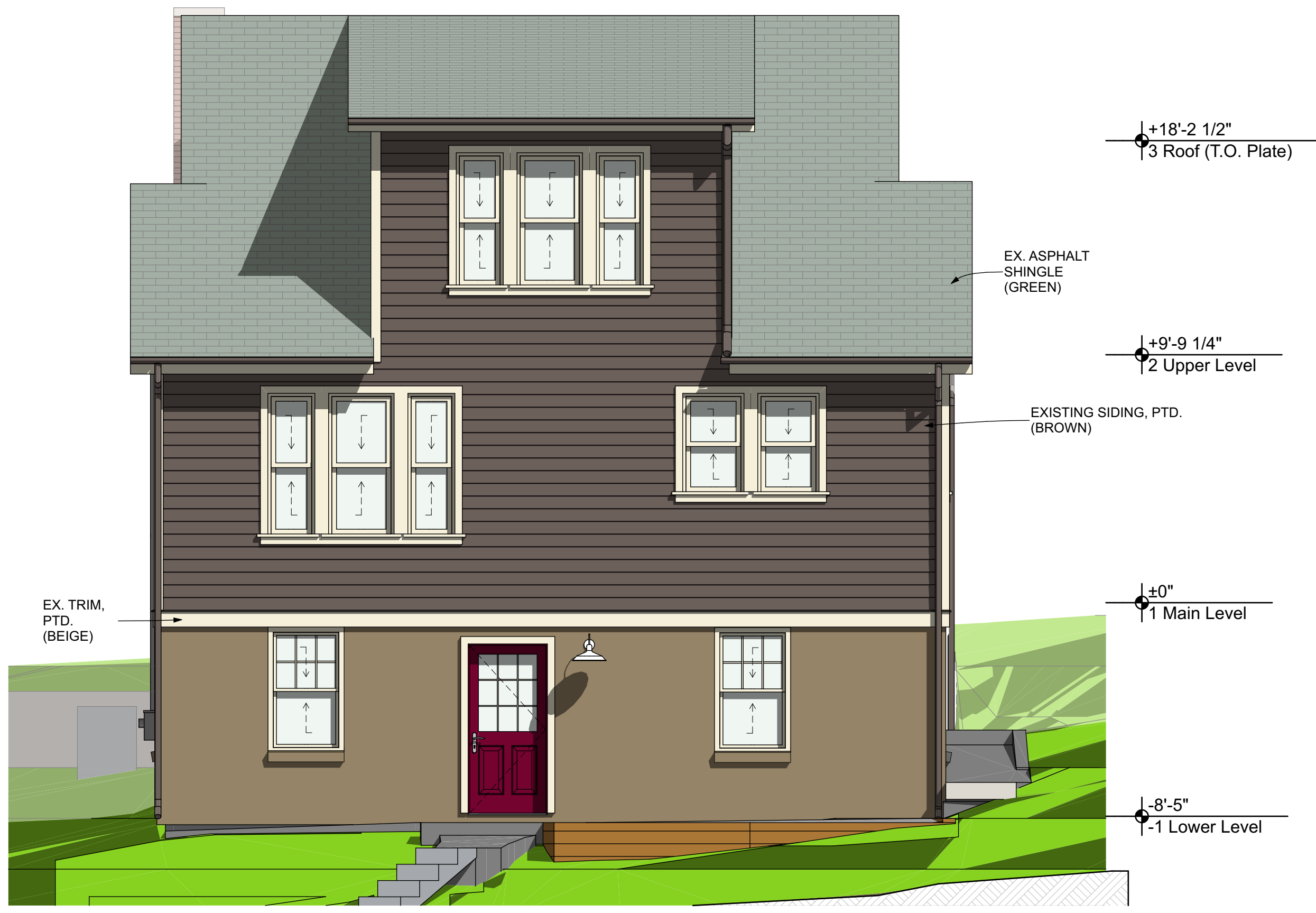
3 North Elevation - EXISTING A008 SCALE: 1/4" = 1'-0"
