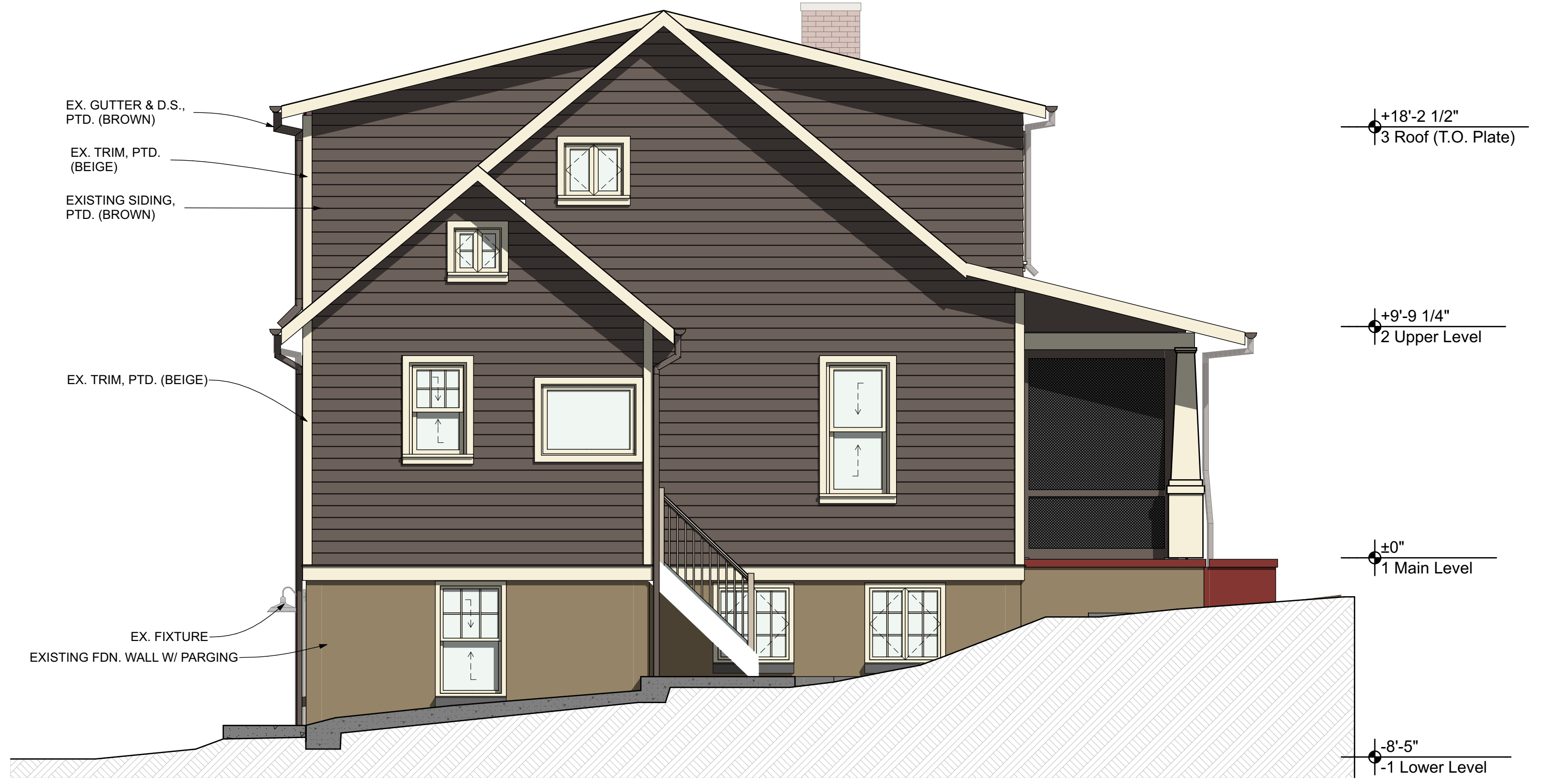
4 West Elevation - EXISTING A008 SCALE: 1/4" = 1'-0"
