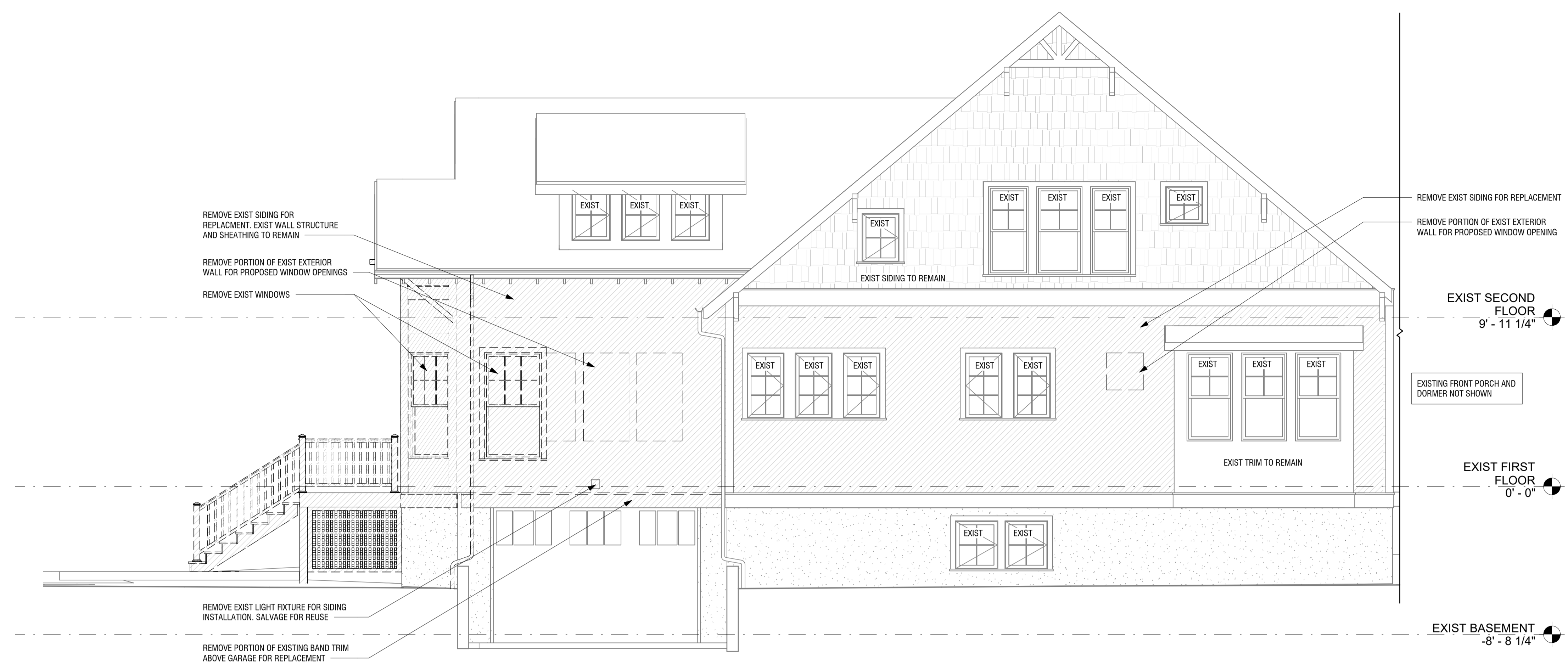
1 SIDE 1 DEMO EXTERIOR ELEVATION 1/4" = 1'-0"
