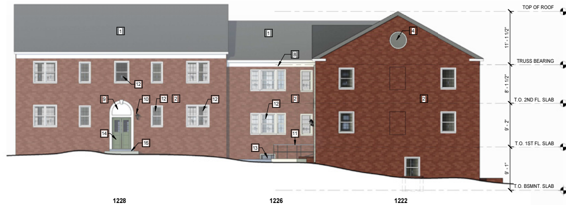
2 BUILDING 14 NORTH ELEVATION 1/8" = 1'-0"
