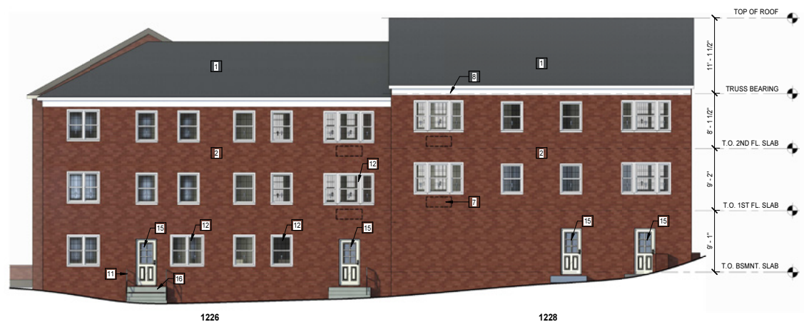
1 BUILDING 14 SOUTH ELEVATION 1/8" = 1'-0"
