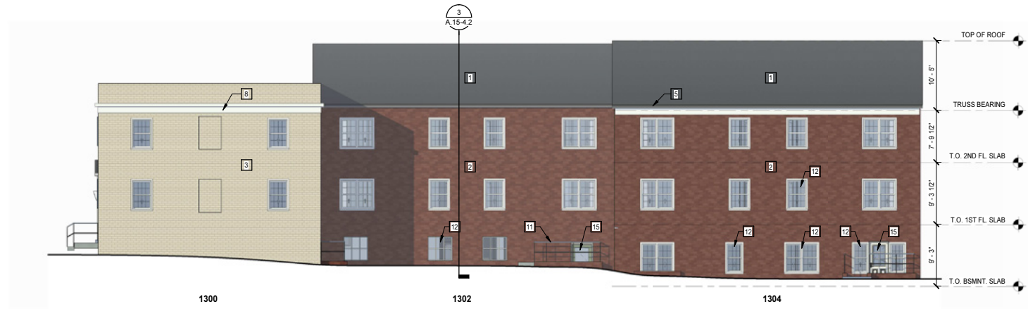
1 BUILDING 15 WEST ELEVATION 1/8" = 1'-0"
