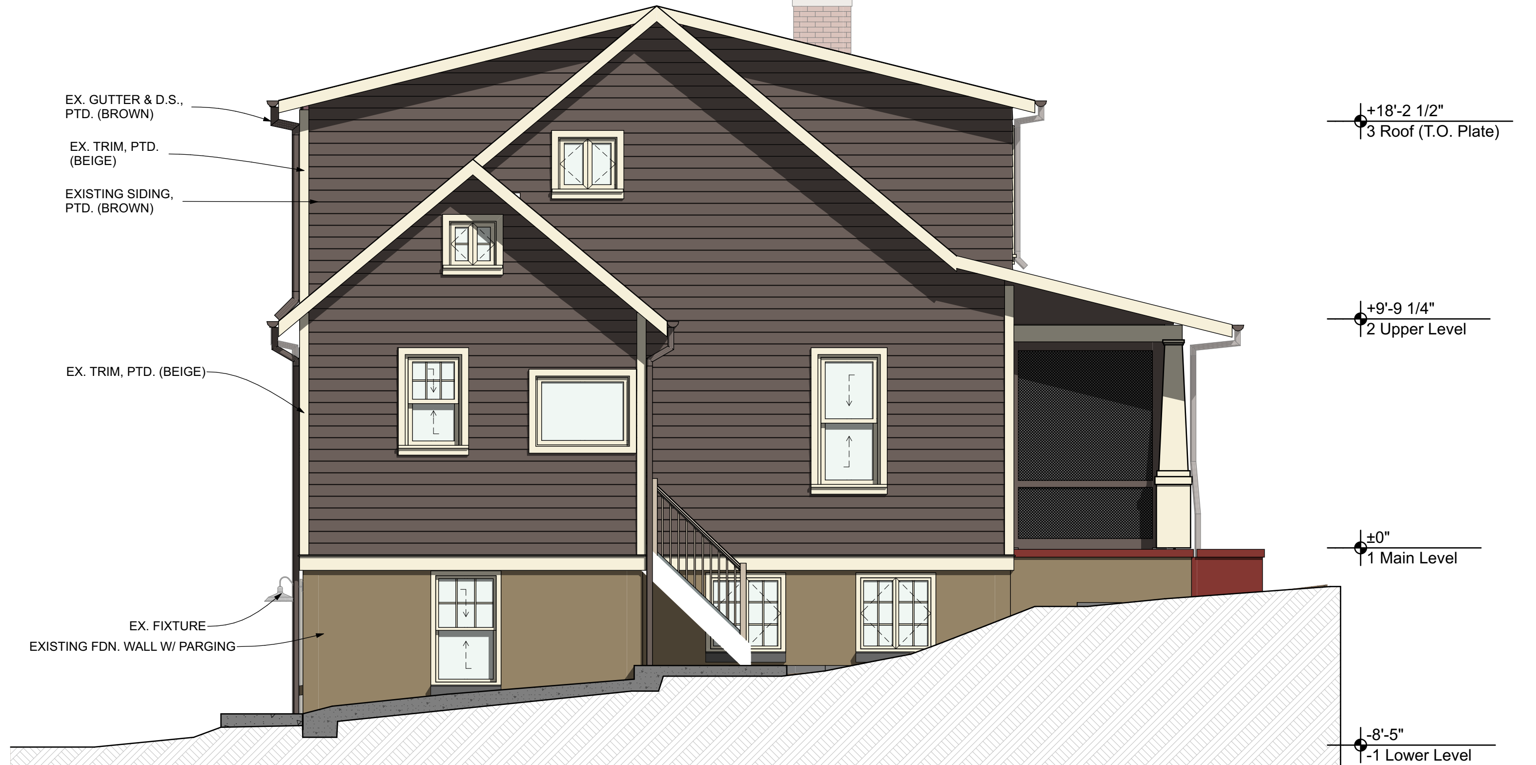
4 West Elevation - EXISTING A008 SCALE: 1/4" = 1'-0"
