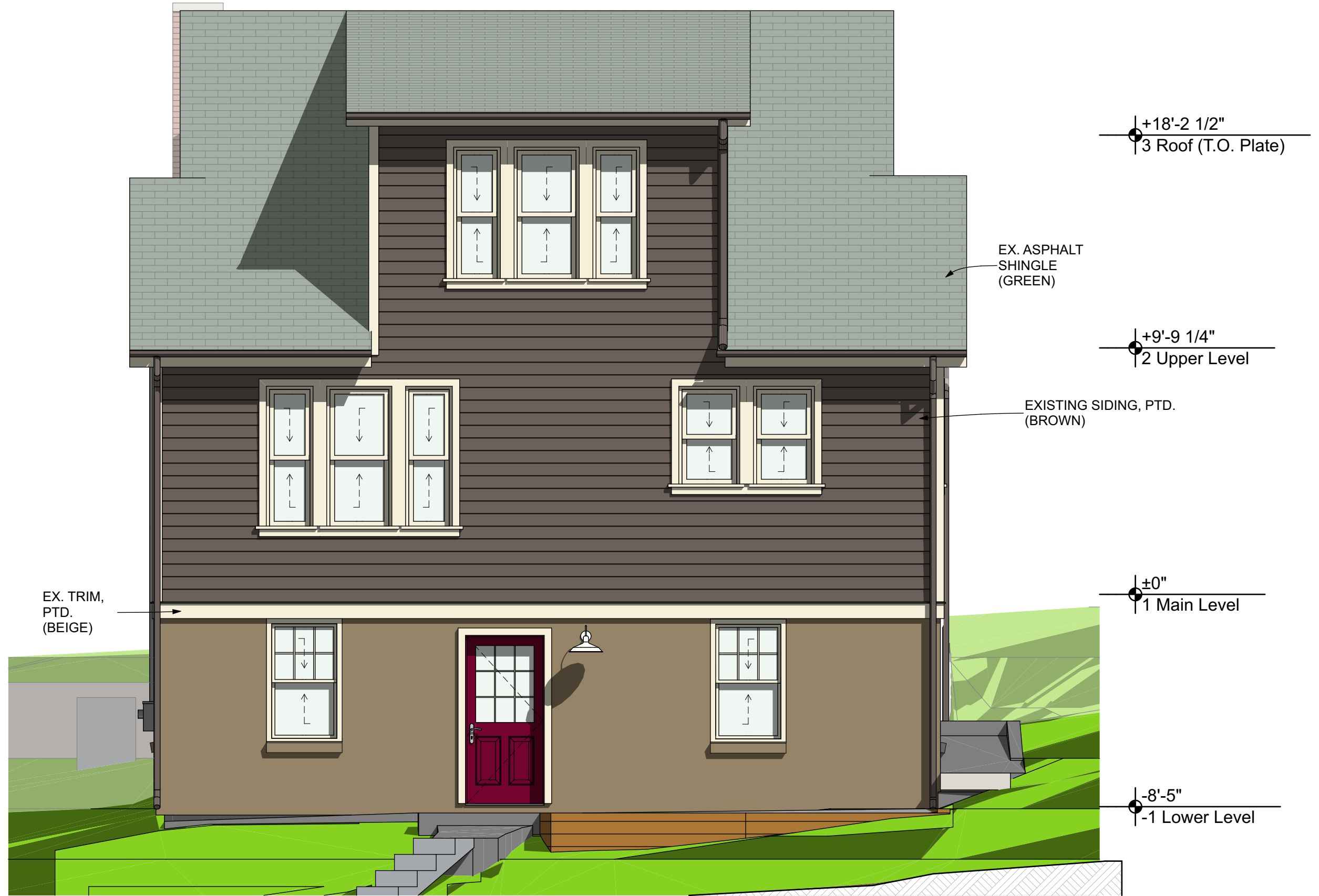
3 North Elevation - EXISTING A008 SCALE: 1/4" = 1'-0"
