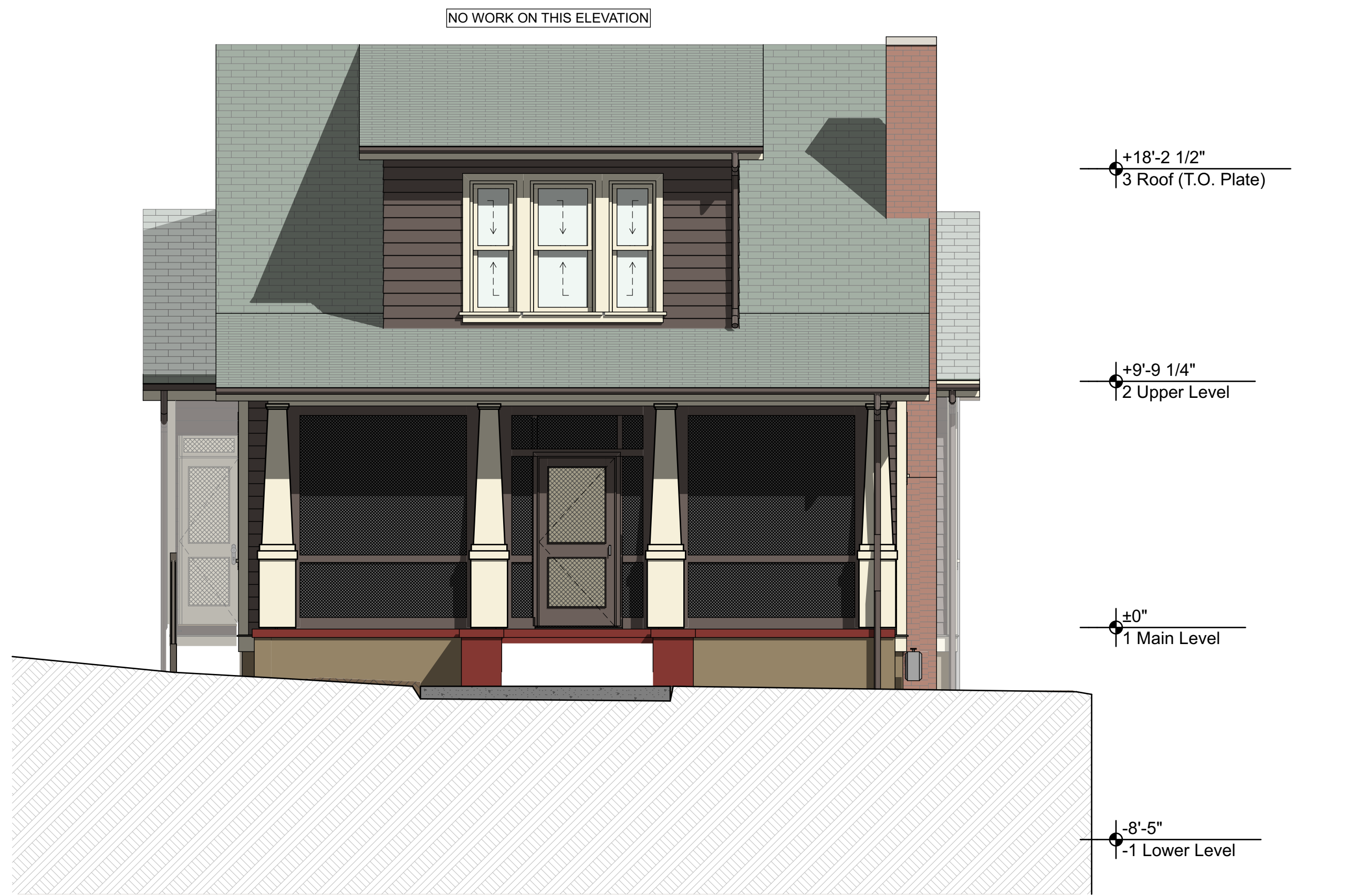
1 South Elevation - EXISTING A008 SCALE: 1/4" = 1'-0"
