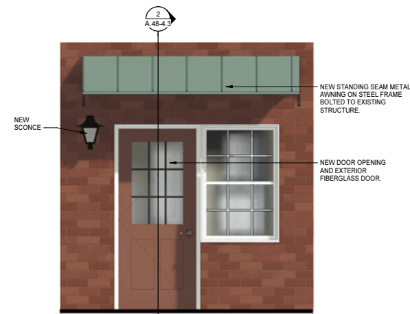
3 BLDG 48 - ENLARGED ELEVATION - ACCESSIBLE ENTRANCE 1 1/2" = 1'-0"
