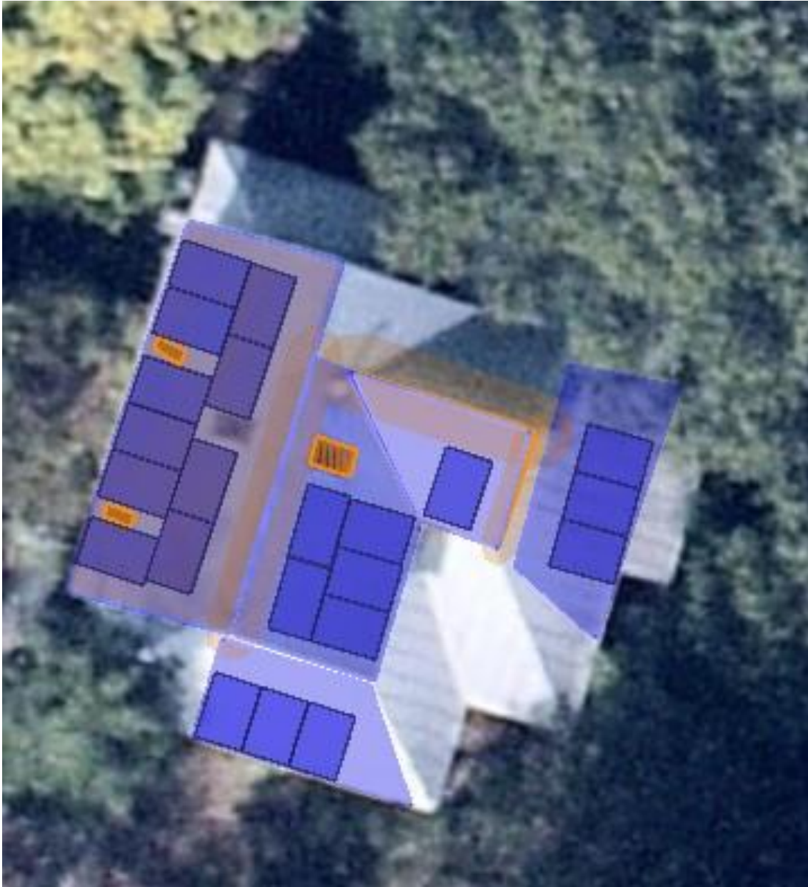
Figure 6: The solar panels are placed in portrait & landscape orientation. Overall, the solar production is good. No shading present on the roof.
