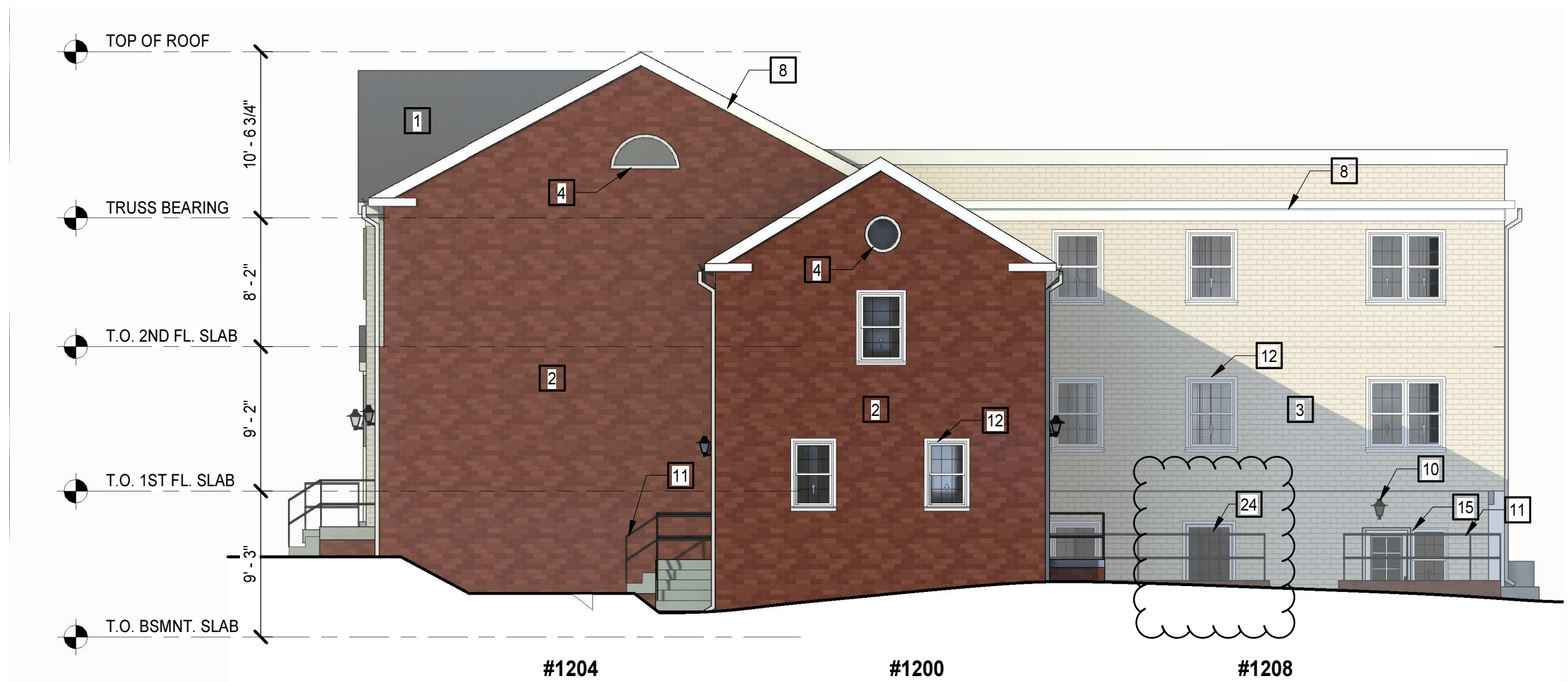
2 BUILDING 12 NORTH ELEVATION 12-A2.0 12-A4.2 1/8" = 1'-0"
