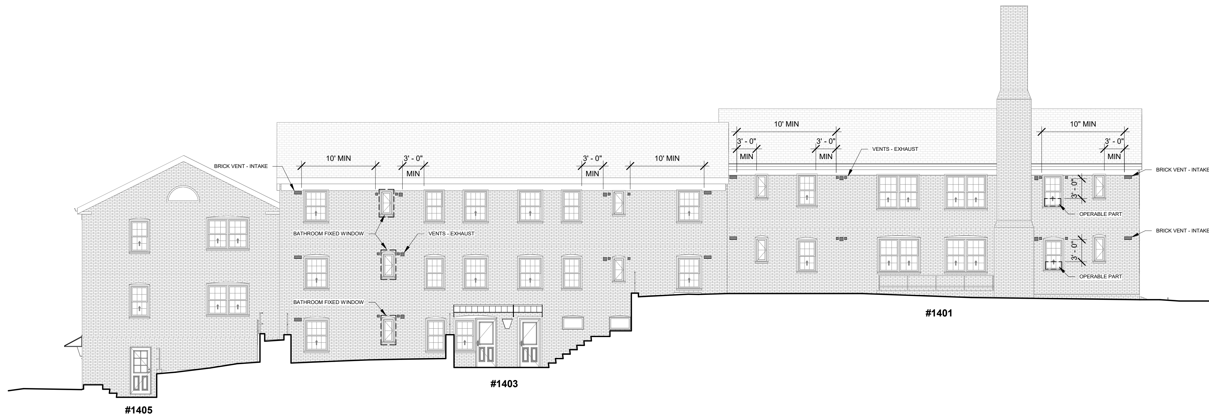
2 A38 TYPICAL PENETRATIONS - BACK FACADE 1/8" = 1'-0"
