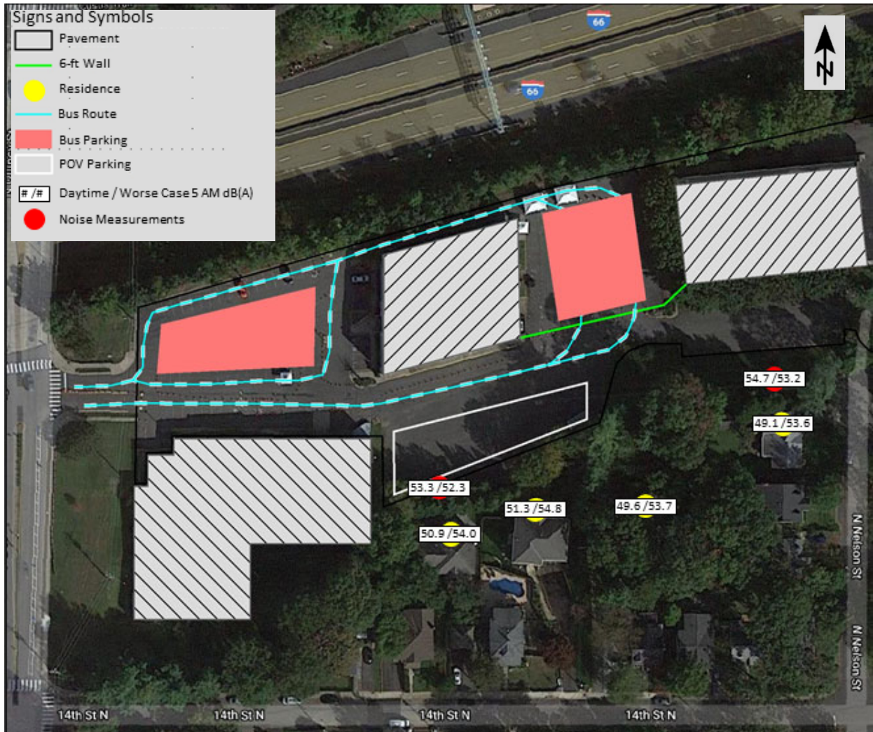
Figure 11: Measured Noise Levels (Average Daytime/5-6am) and Predicted (Daytime/Worst Case) Noise Levels with Abatement
