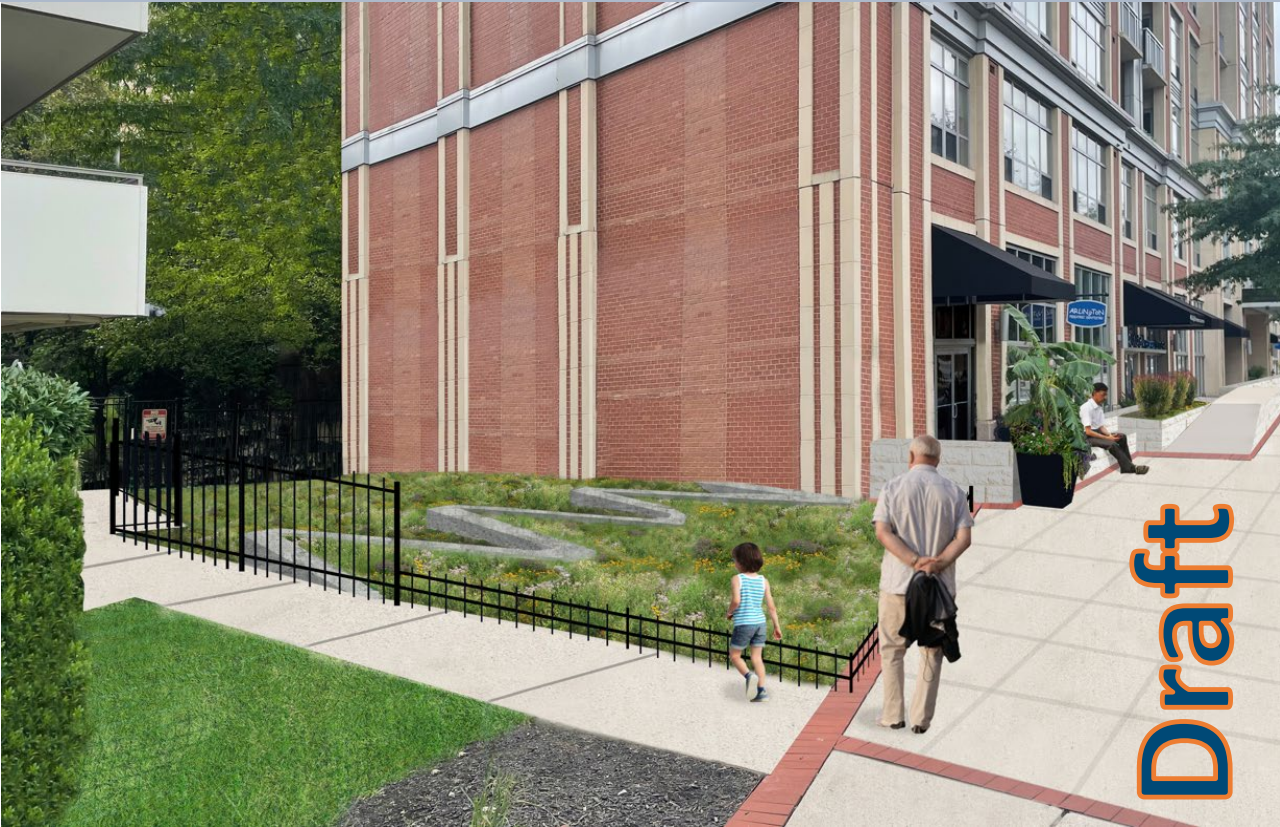
2.5' concrete seat wall protects against 5- to 10-year storm
