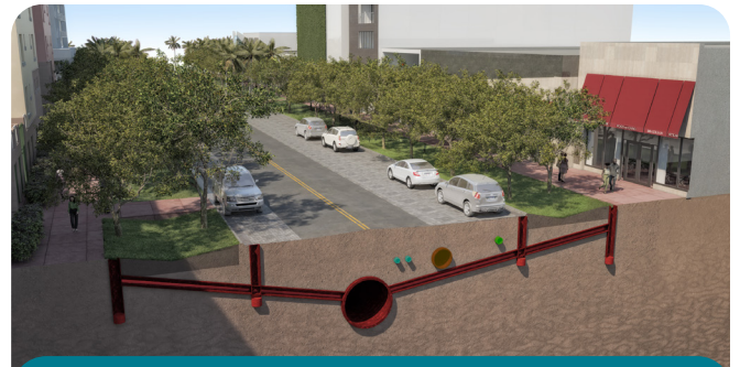
Figure 2 - Example street cross-section showing stormwater inlets, pipes, other utilities, and a larger conveyance pipe
