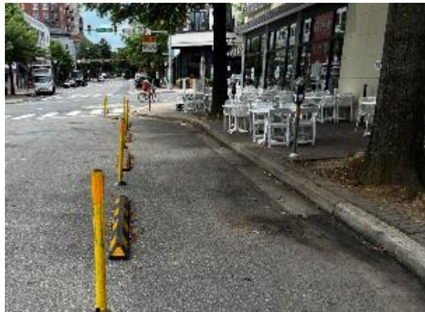
Examples of TOSAs that utilized the entire sidewalk with pedestrian circulation temporarily relocated in the on-street parking area.
