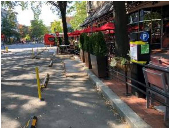
Examples of TOSAs that utilized the entire sidewalk with pedestrian circulation temporarily relocated in the on-street parking area.
