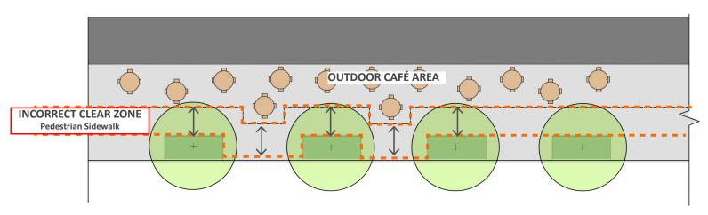
The Clear Zone must be a straight path. The Clear Zone cannot zigzag or be measured from varied obstruction points along the pedestrian path.
