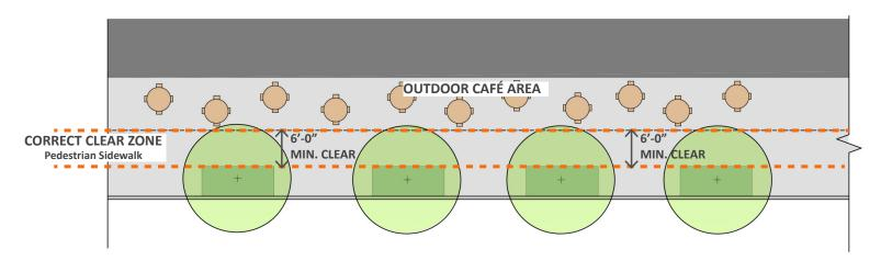
The Clear Zone is measured in a consistently straight path from the closest obstructions on both sides. Six feet minimum must be left clear for pedestrians. Site Plan Conditions or Sector Plans may call for a wider clear zone.
