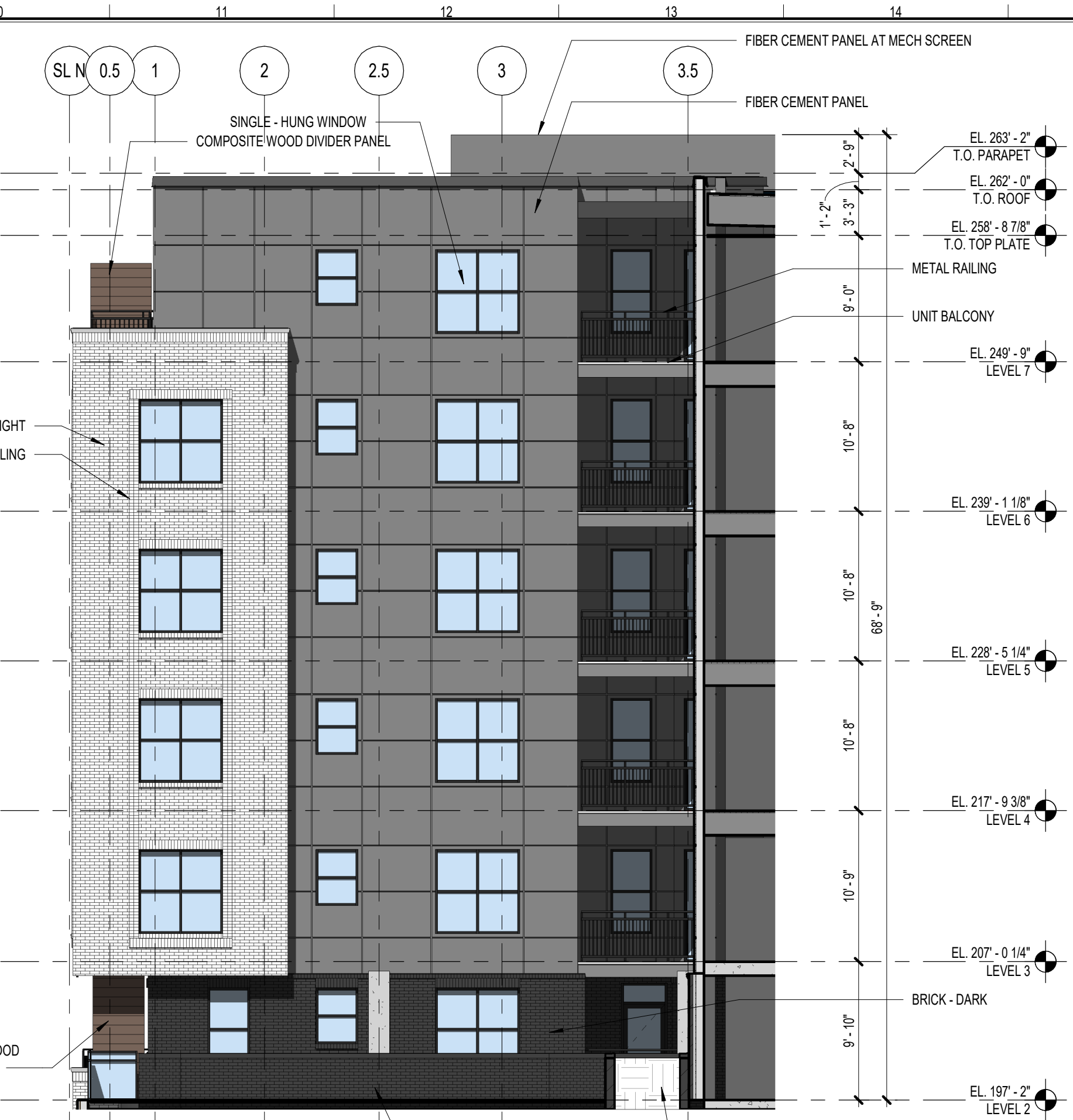
3 ZA-BLDG. ELEVATION WEST - NORTH COURTYARD A-04.05 SCALE: 1/8" = 1'-0"
