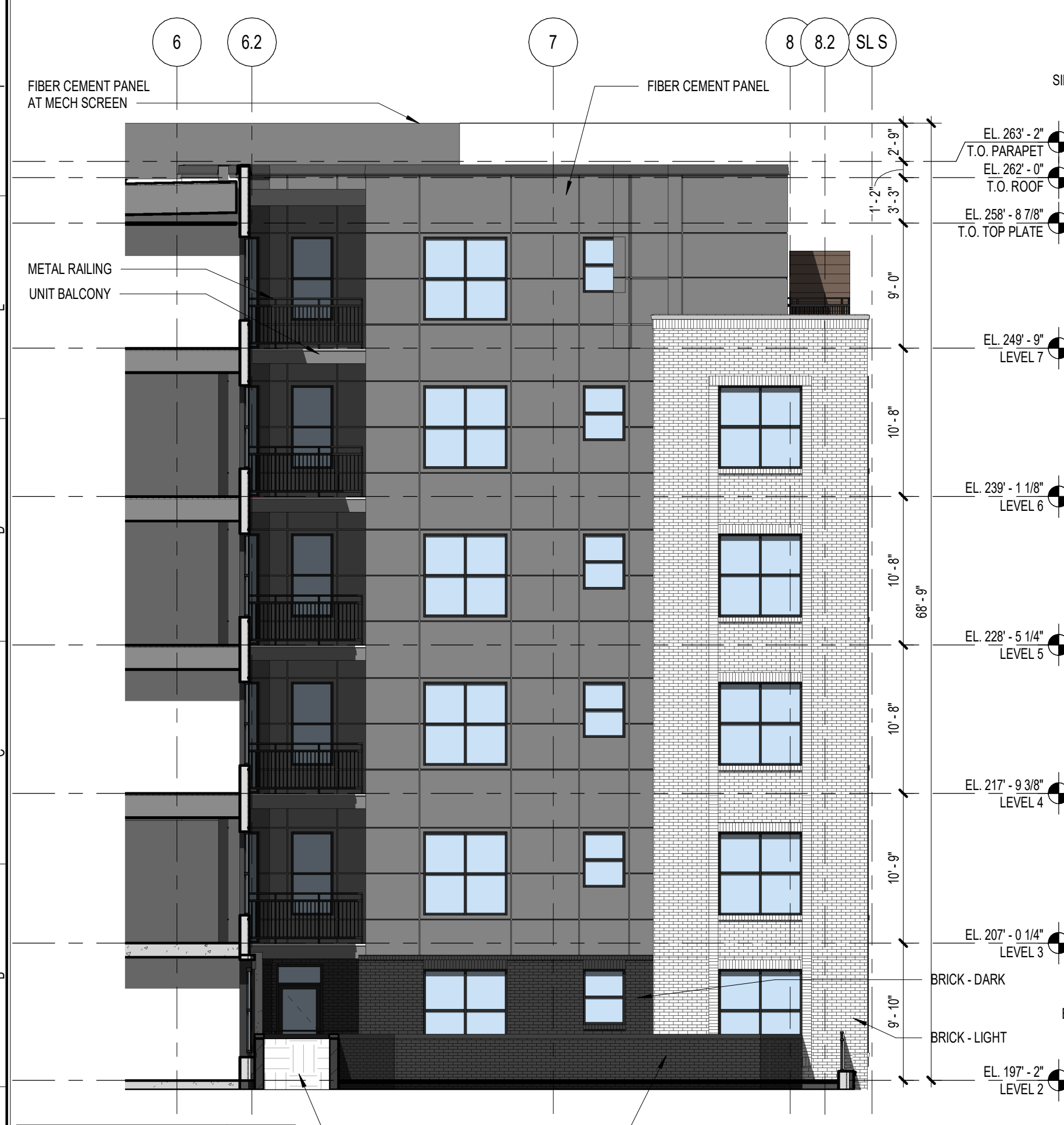
4 ZA-BLDG. ELEVATION WEST - SOUTH COURTYARD A-04.05 SCALE: 1/8" = 1'-0"
