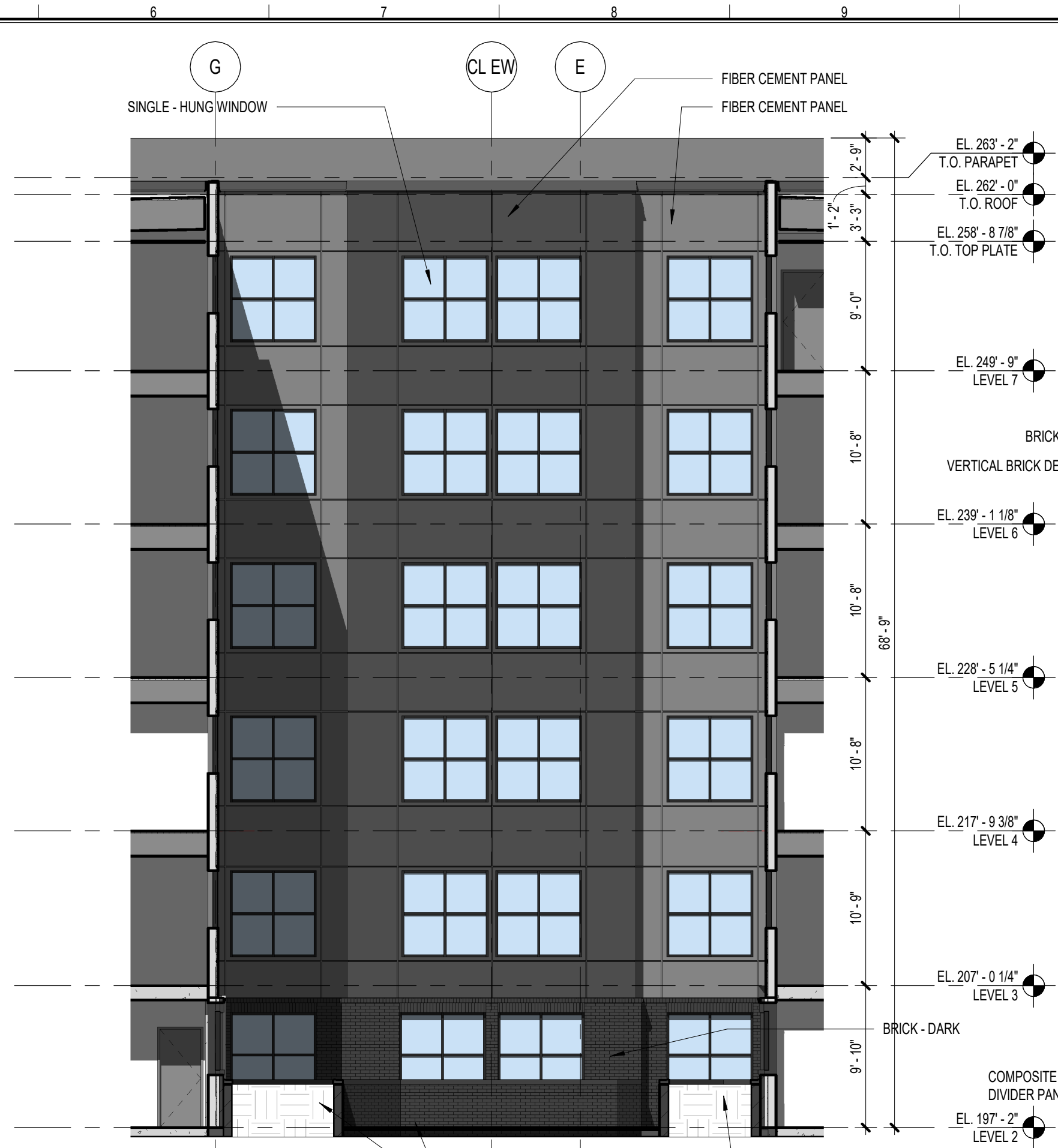
2 ZA-BLDG. ELEVATION NORTH - NORTH COURTYARD A-04.05 SCALE: 1/8" = 1'-0"
