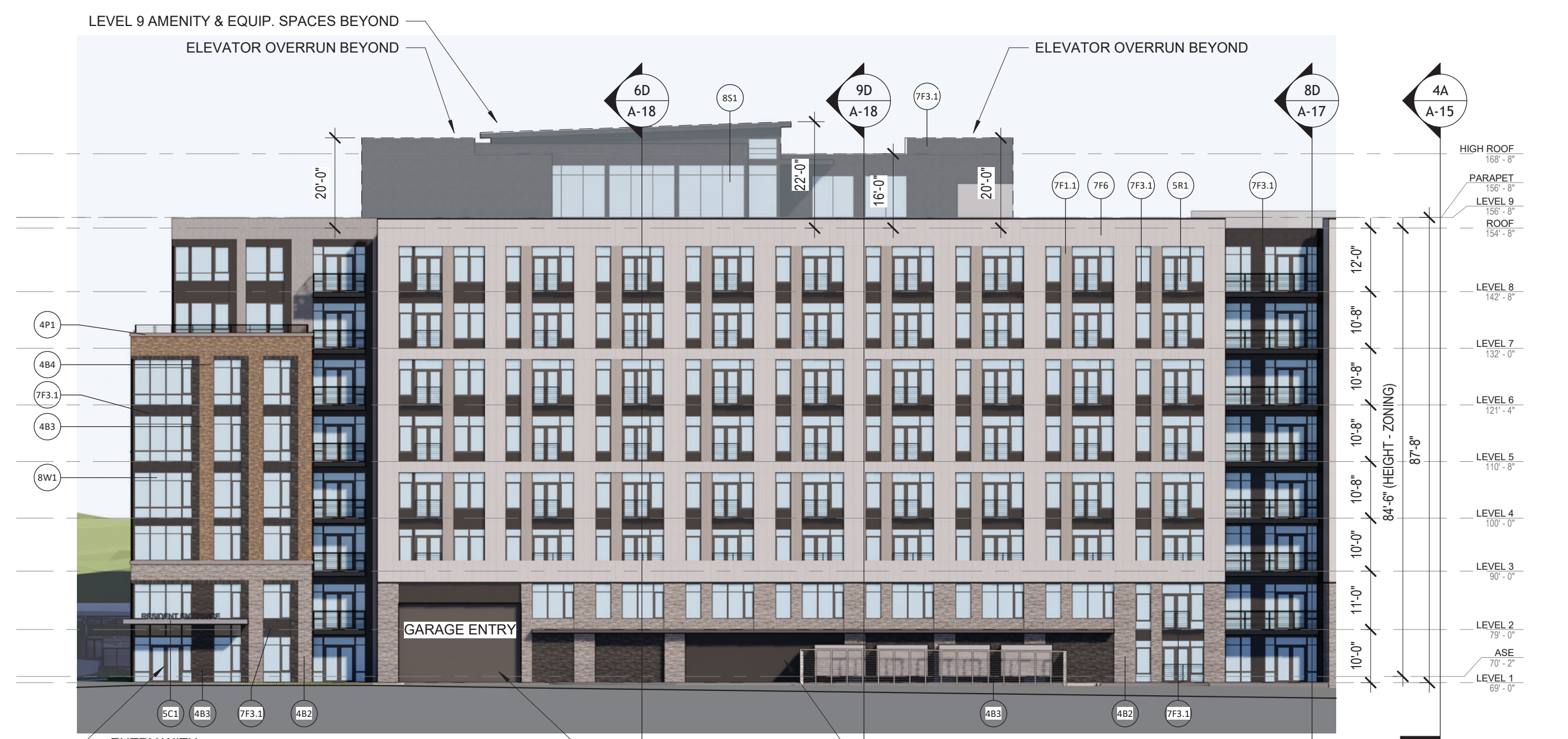
7A BUILDING E - SOUTH ELEVATION 1 A-02 A-21 1" = 20'-0"
