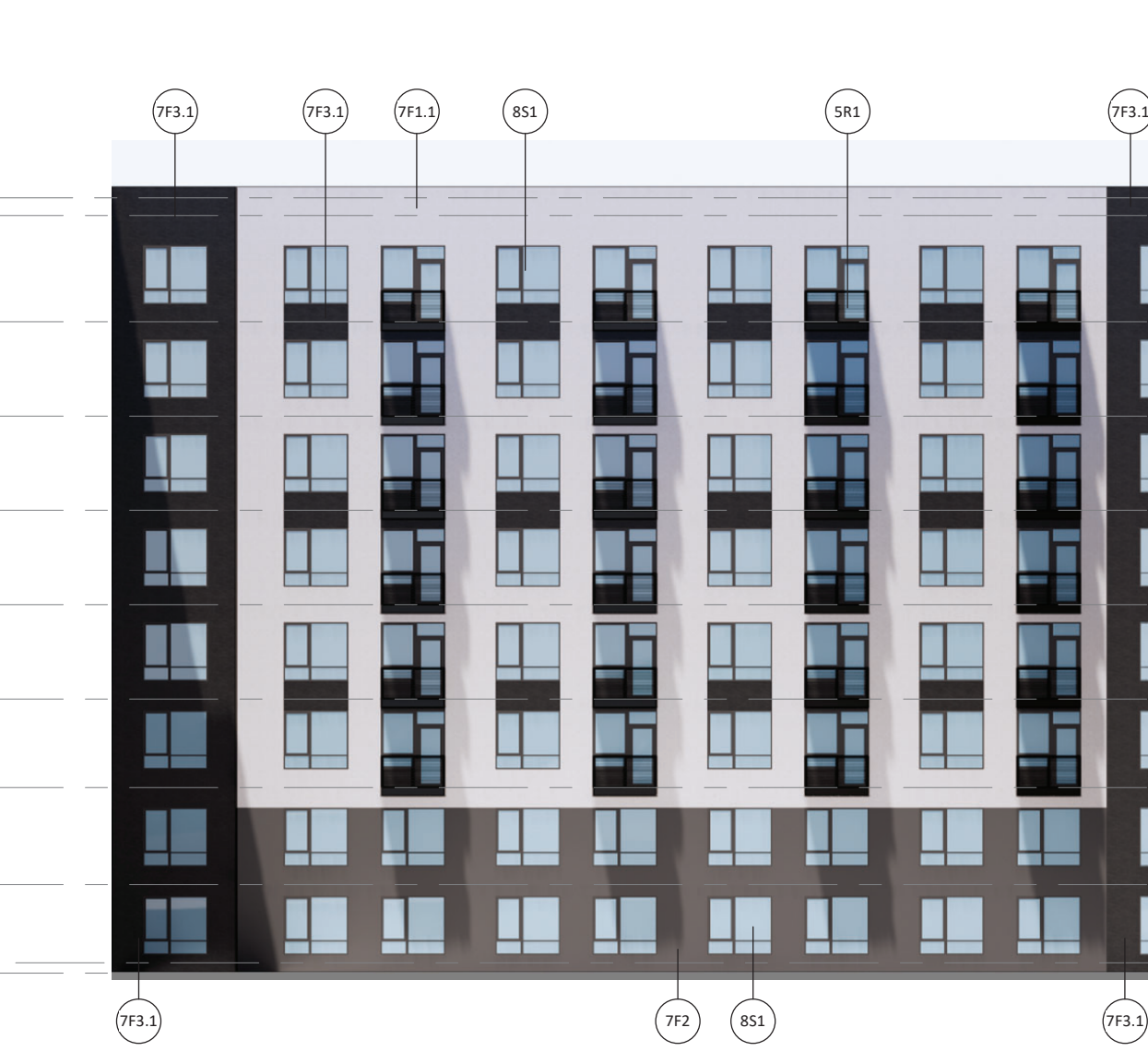
7D BUILDING E - COURTYARD SOUTH ELEVATION A-02 A-22 1" = 20'-0"
