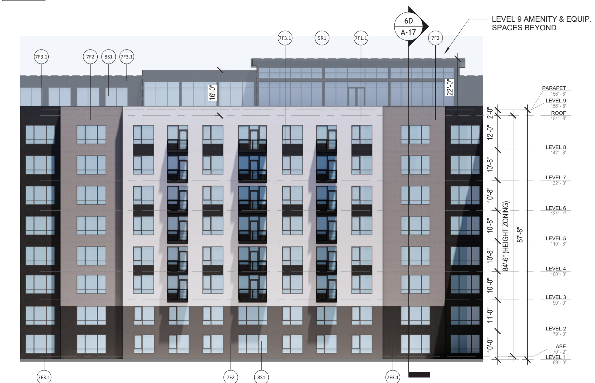
5A BUILDING E - COURTYARD WEST ELEVATION A-02 A-22 1" = 20'-0"
