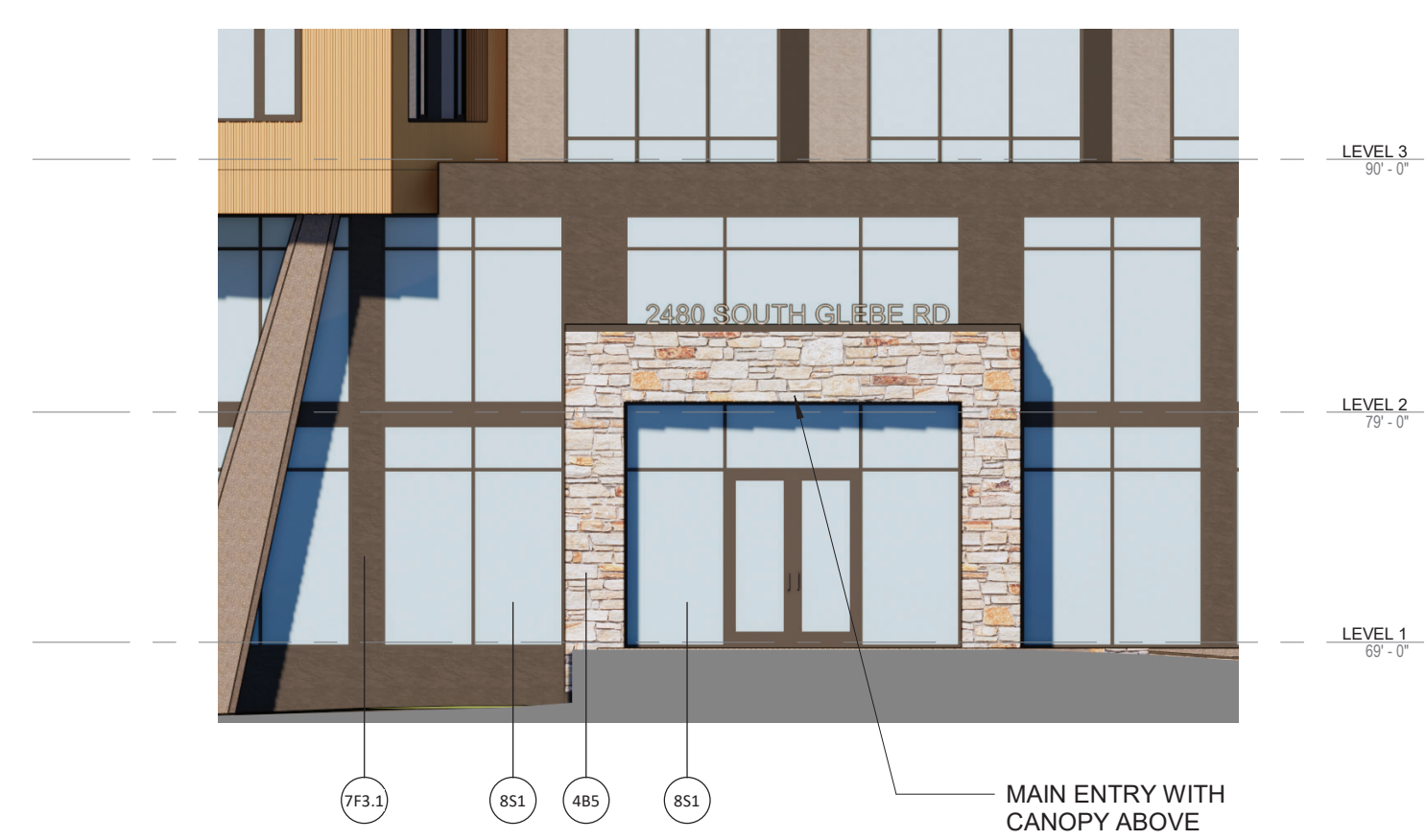
4 --- BLDG E - LEVEL 2 ENTRANCE ENLARGED ELEVATION
