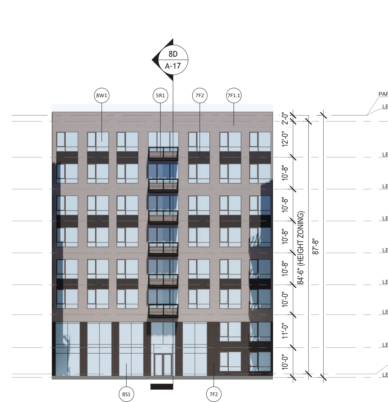
5D BUILDING E - COURTYARD NORTH ELEVATION A-02 A-22 1" = 20'-0"
