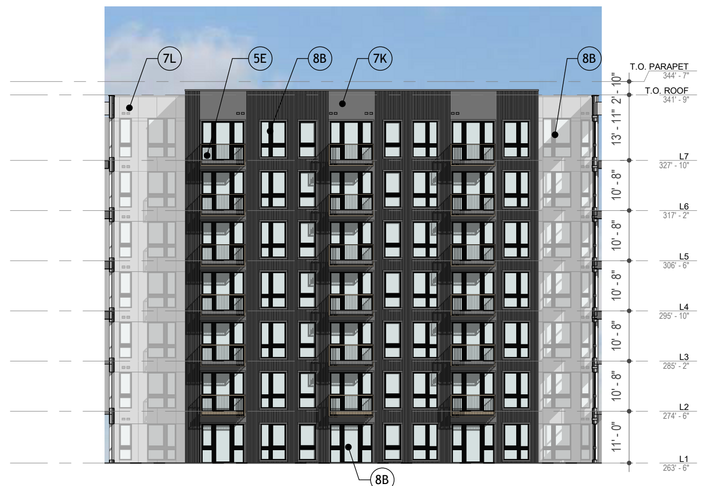
4G COURTYARD - SOUTH ELEVATION A1 A-32 1" = 20'-0"
