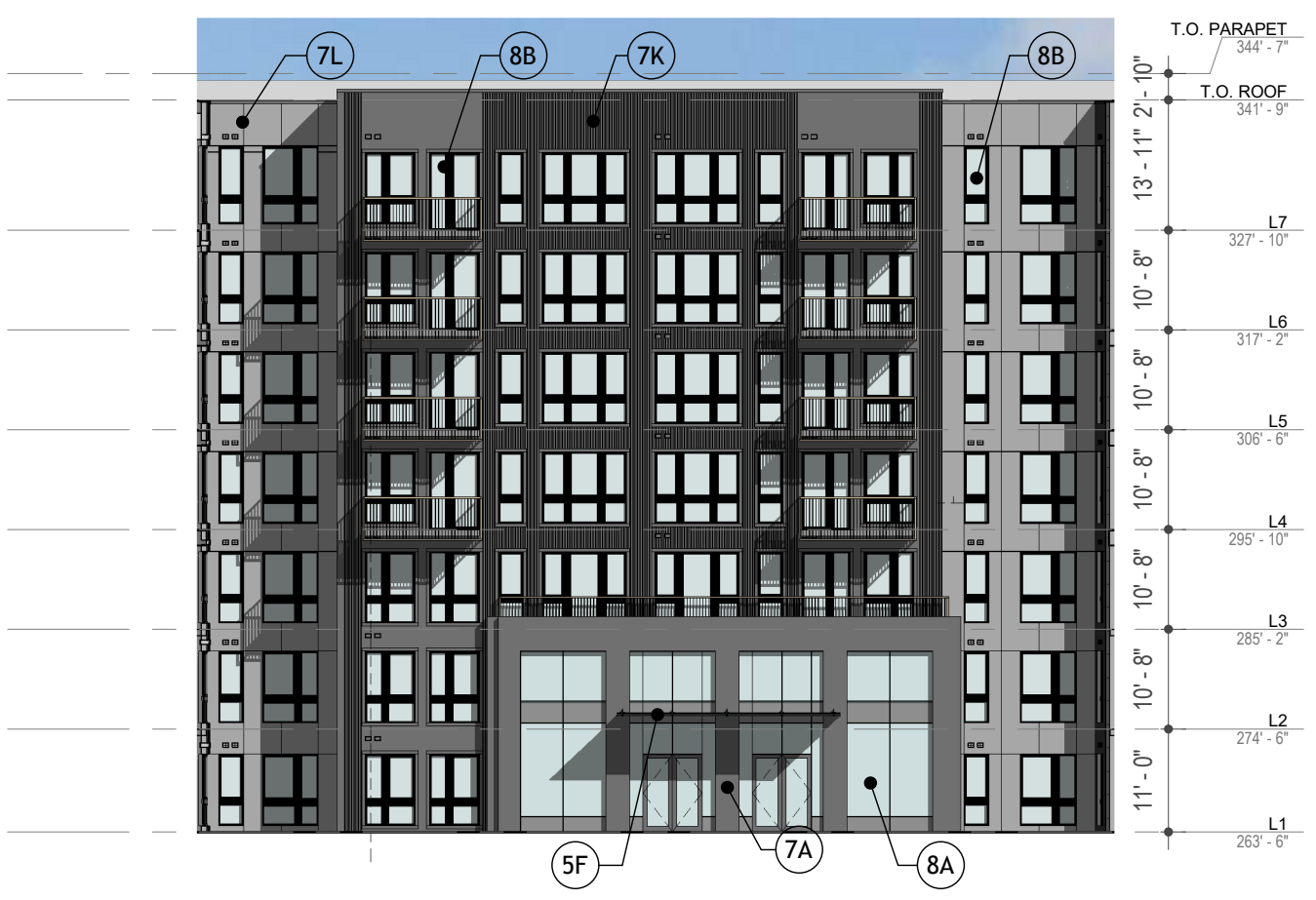
6G COURTYARD - NORTH ELEVATION A1 A-32 1" = 20'-0"
