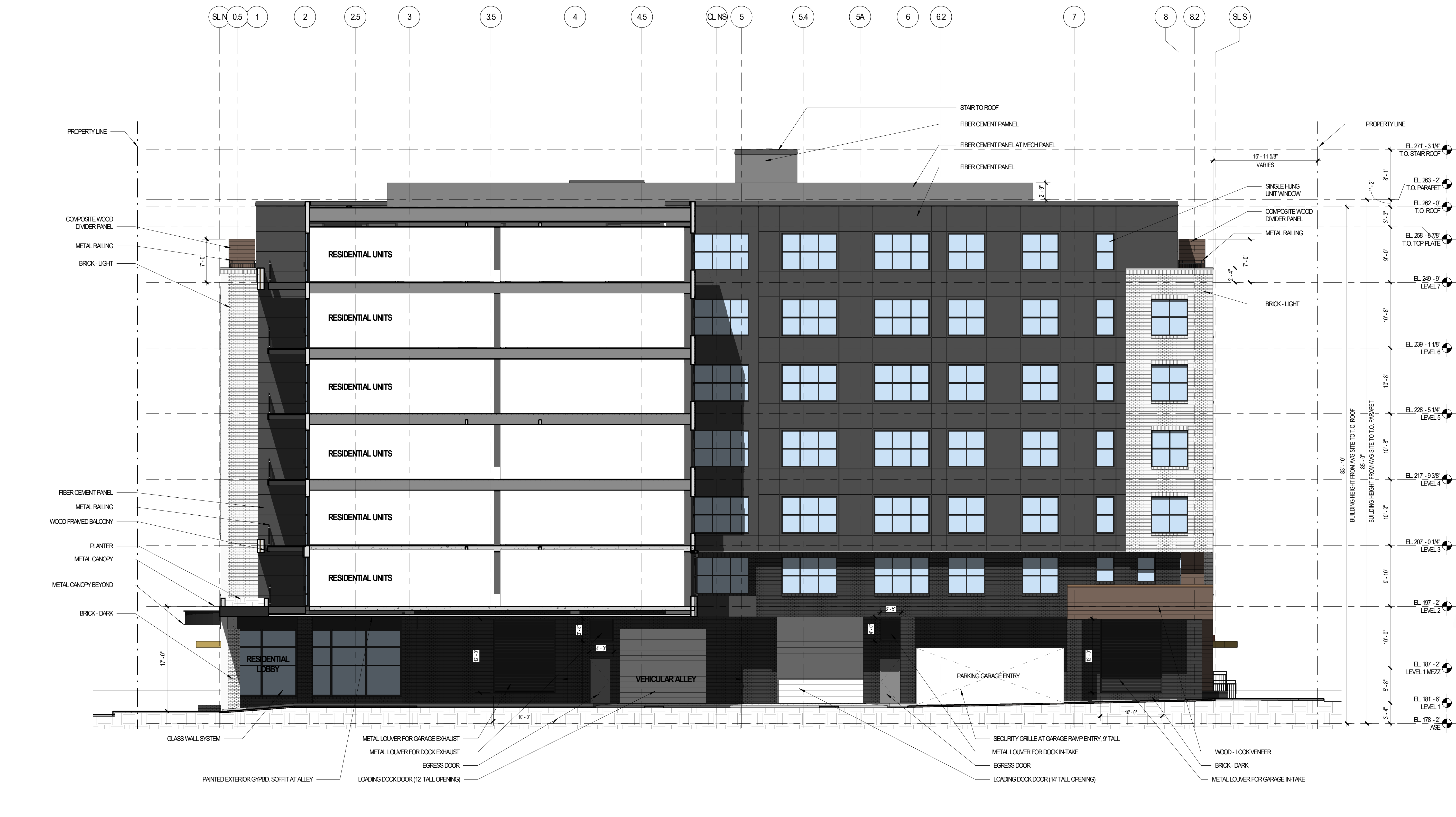
1 ZA-BUILDING ELEVATION WEST AT ALLEY A-04.04 SCALE: 1/8" = 1'-0"
