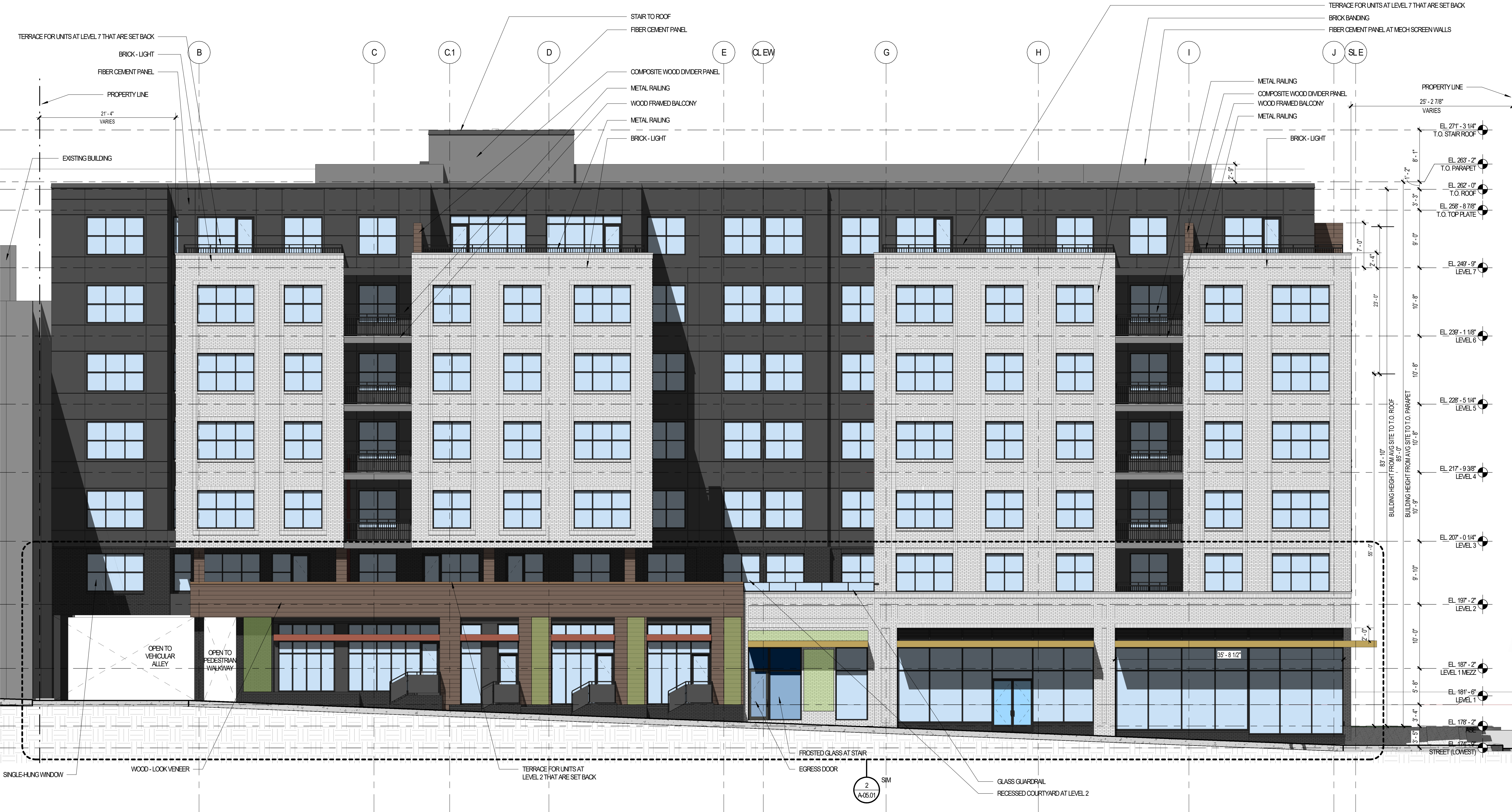
1 A01.08/A-04.01 ZA-BUILDING ELEVATION SOUTH SCALE: 1/8" = 1'-0"
