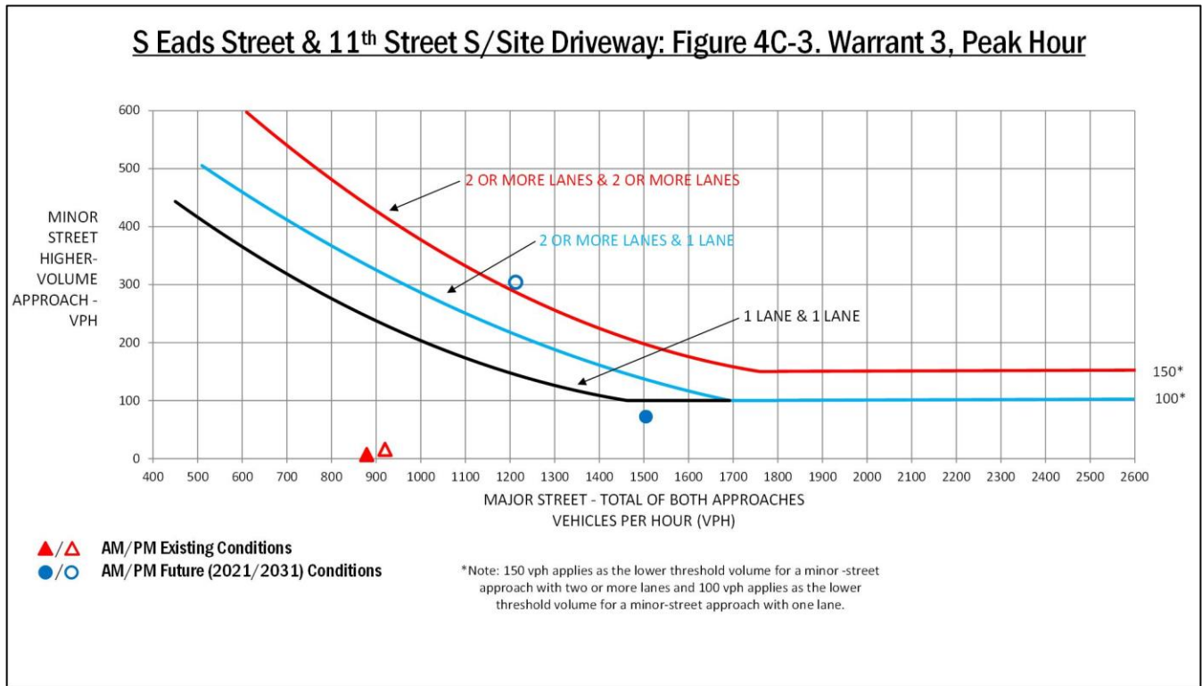
Figure 69: Warrant 3, Peak Hour Vehicle Volume – S Eads Street and 11 th Street S/Site Driveway
