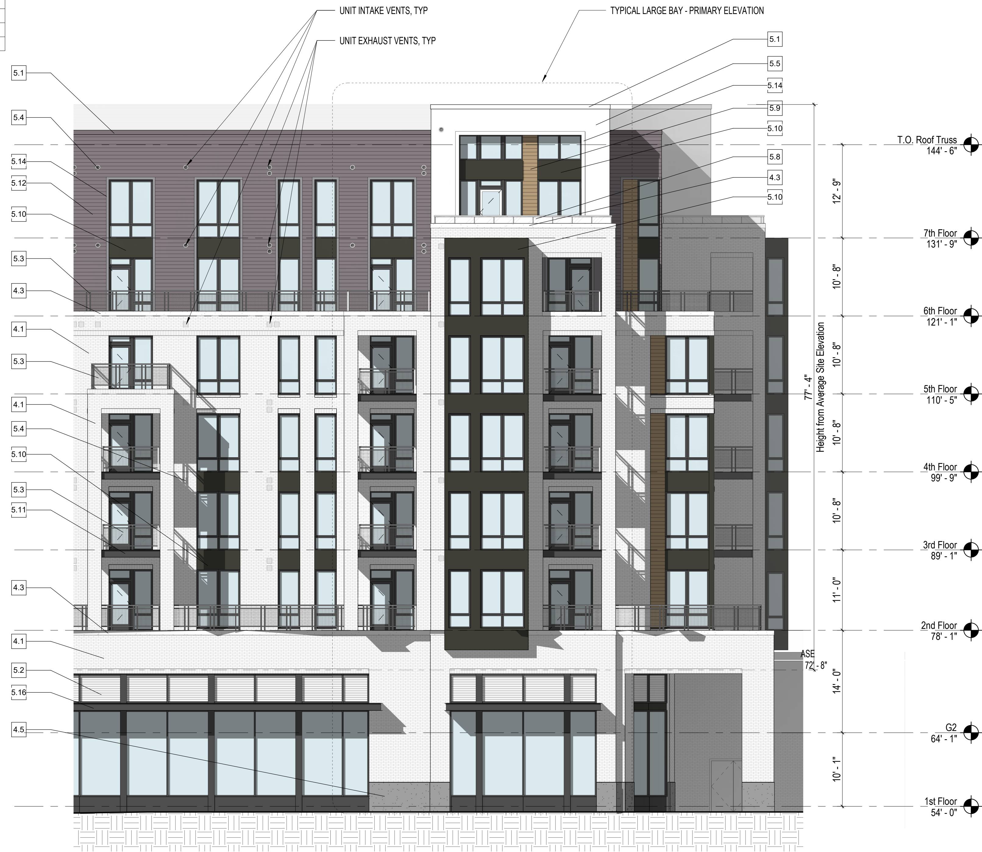
1 Typical Bay Elevation 1/8" = 1'-0"
