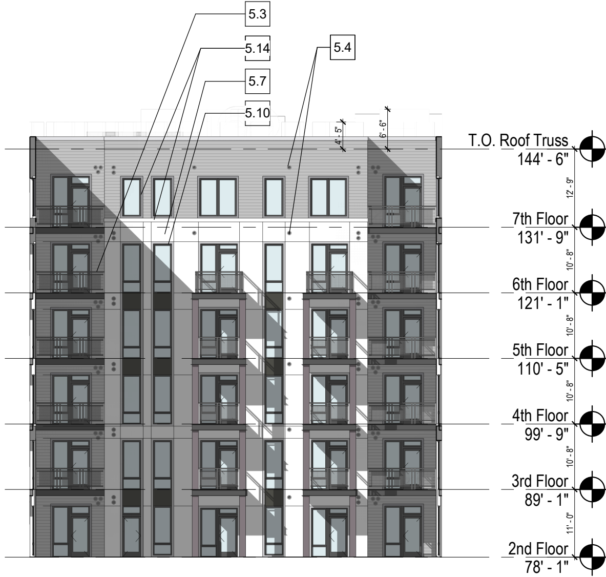
5 BLDG N1 - Courtyard 1 N Elevation 1/16" = 1'-0"
