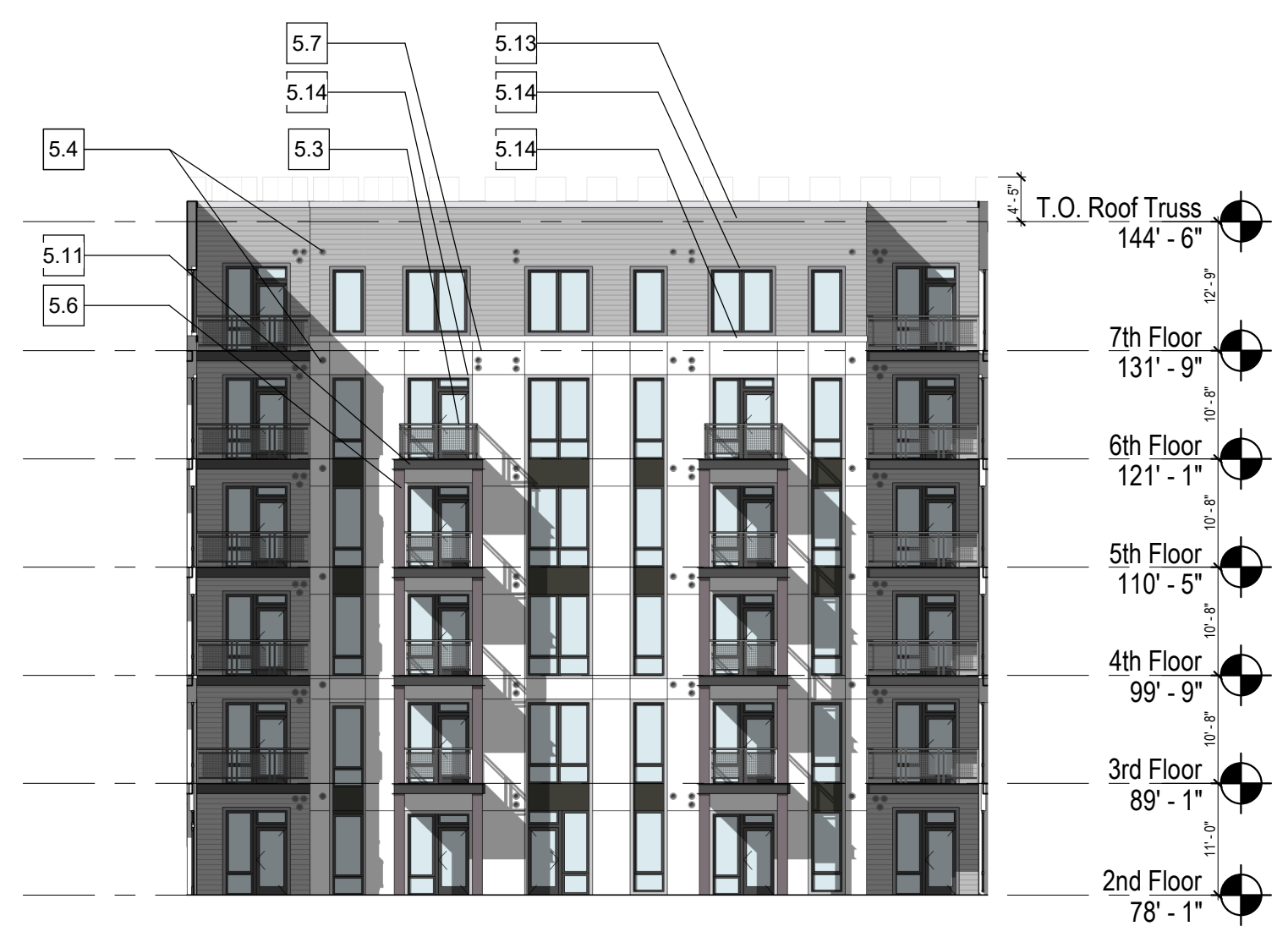
3 BLDG N2 - Courtyard 1 W Elevation 1/16" = 1'-0"
