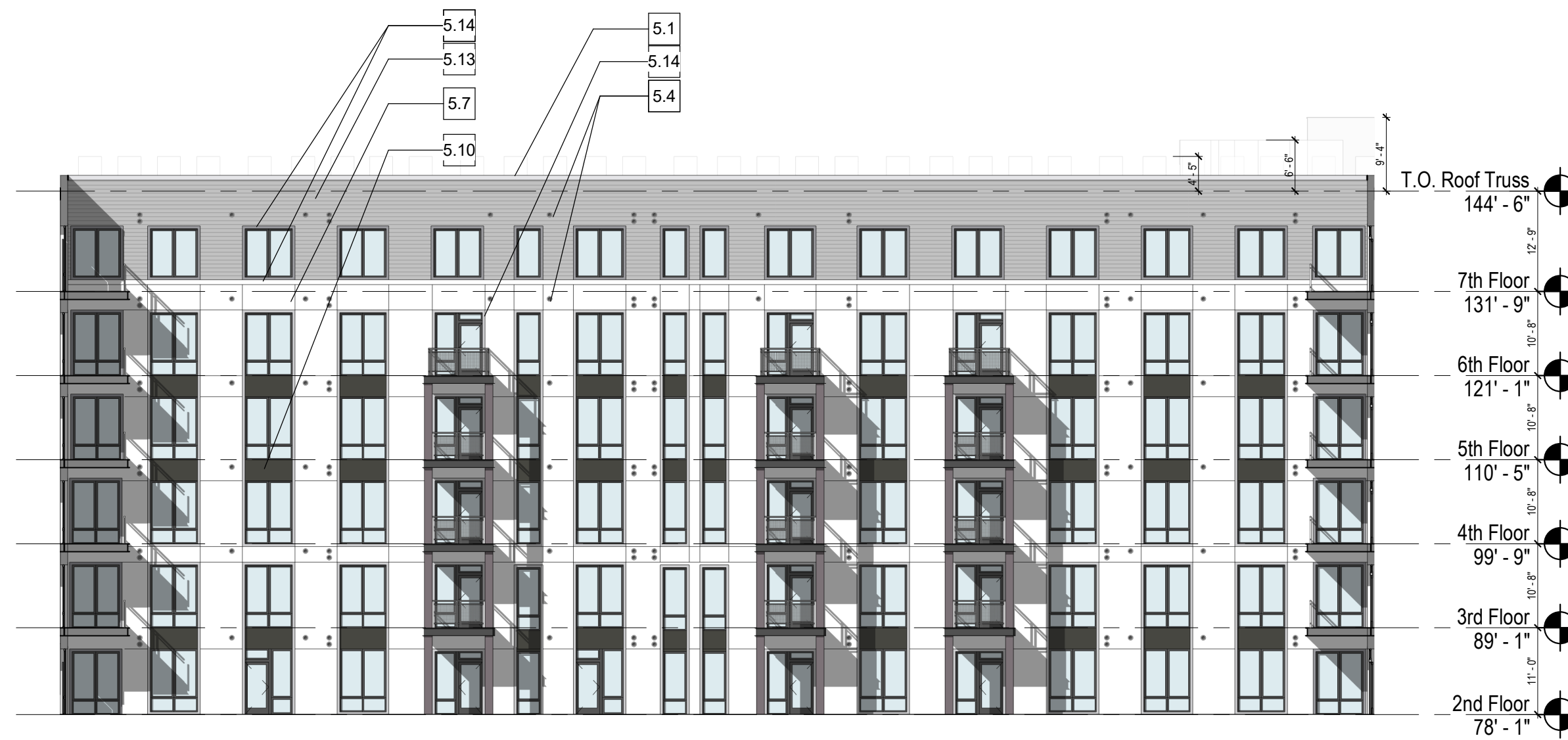
6 BLDG N1 - Courtyard 1 W Elevation 1/16" = 1'-0"
