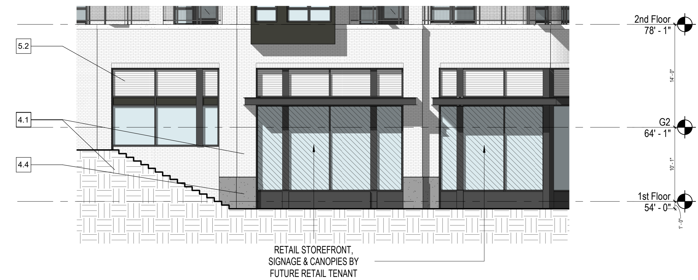
2 Enlarged Elevation - BLDG N2 Retail Entrance 1/8" = 1'-0"
