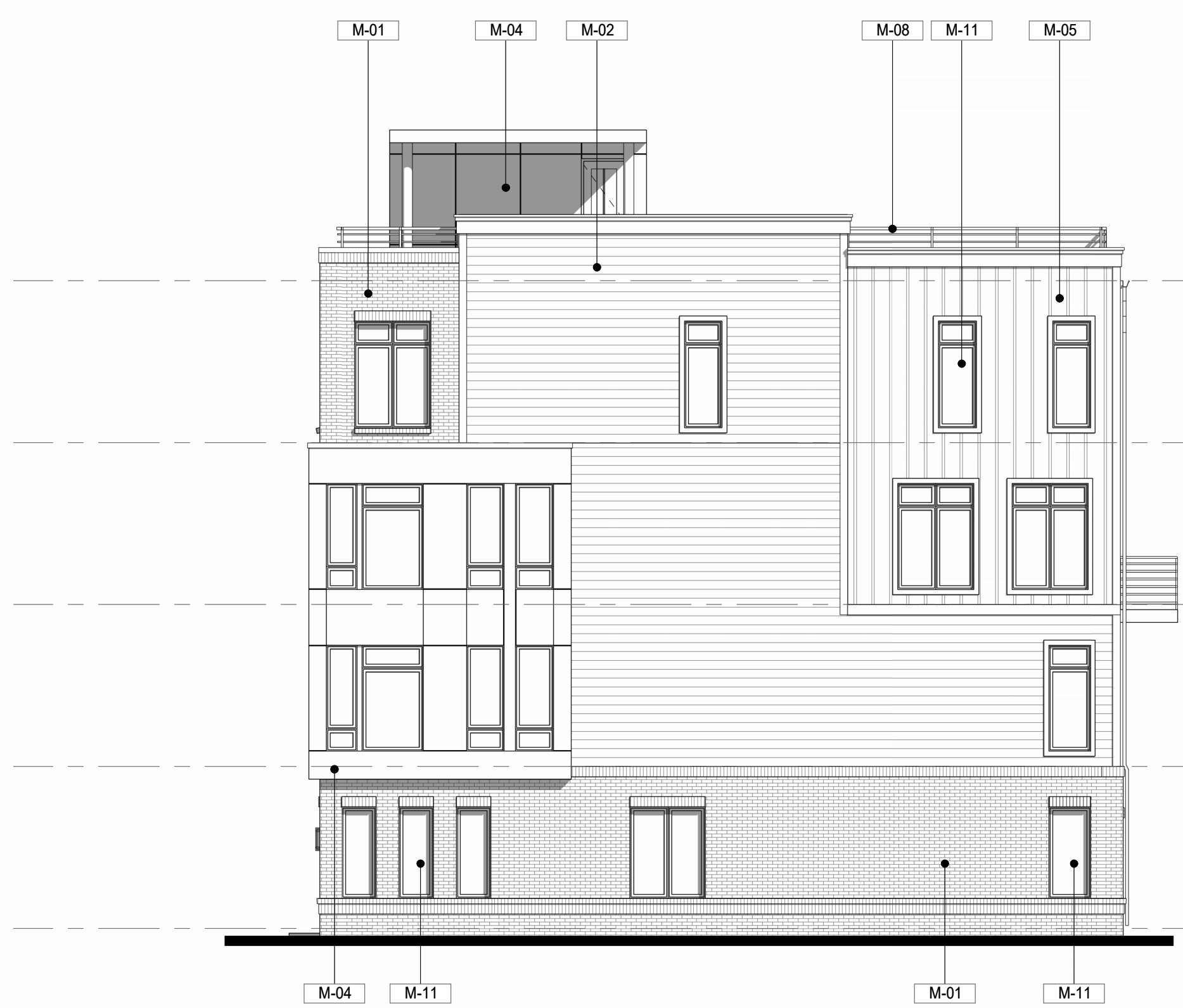
2 SIDE ELEVATION - LV A.S-103 1/8" = 1'-0" WALL OPENING:17%
