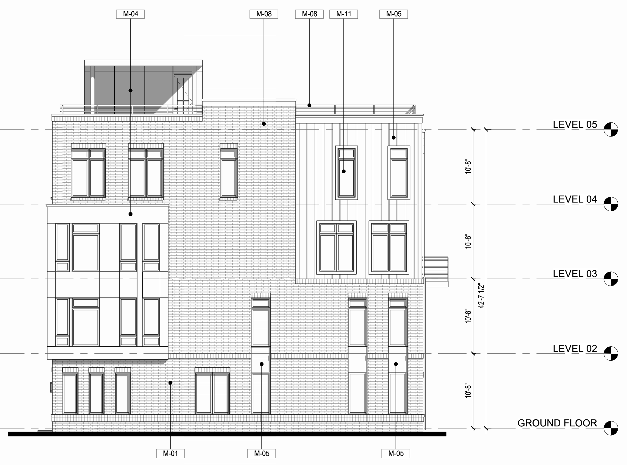
1 SIDE ELEVATION - HV A.S-103 1/8" = 1'-0" WALL OPENING:22%
