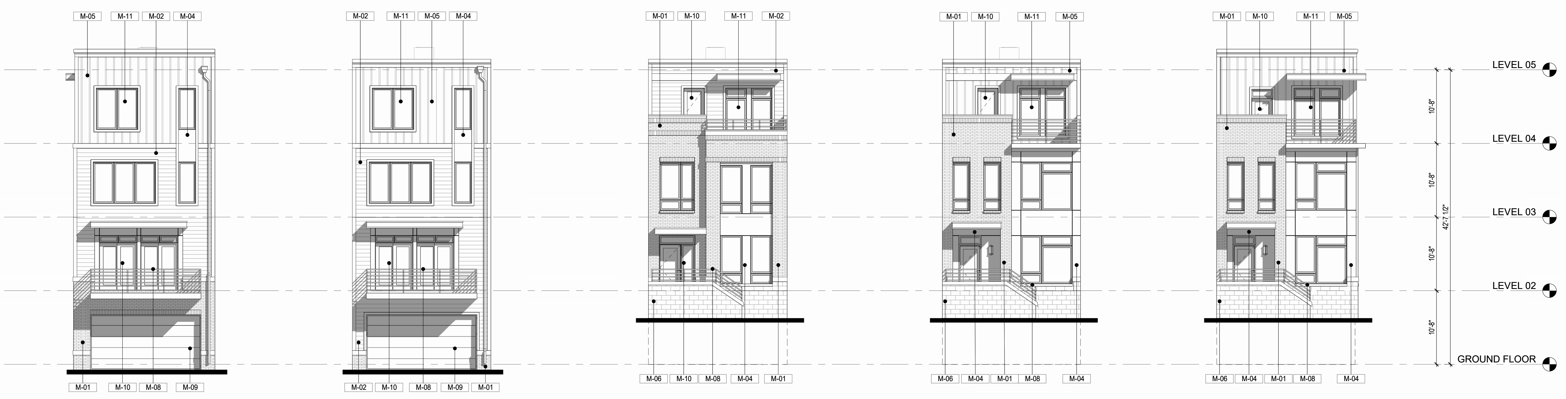
5 REAR ELEV. - END HV A.S-112 1/8" = 1'-0" WALL OPENING:36% 4 REAR ELEV. - INT A.S-112 1/8" = 1'-0" WALL OPENING:38% 3 FRONT - ELEV. #2 INT. A.S-112 1/8" = 1'-0" WALL OPENING:27% 2 FRONT - ELEV. #1 INT. A.S-112 1/8" = 1'-0" WALL OPENING:27% 1 FRONT - ELEV. #1 END A.S-112 1/8" = 1'-0" WALL OPENING:30%
