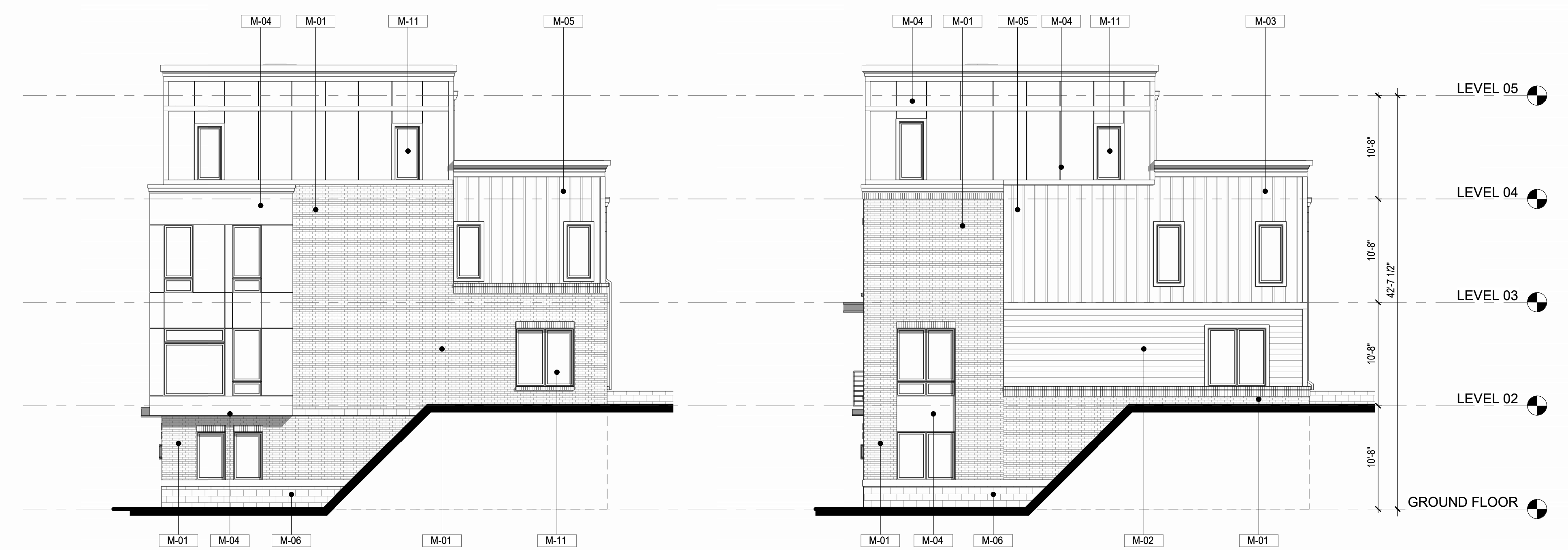
5 SIDE ELEVATION - HIGH VIS A.S-133 1/8" = 1'-0" WALL OPENING:12% 4 SIDE ELEVATION - LOW VIS A.S-133 1/8" = 1'-0" WALL OPENING:9%
