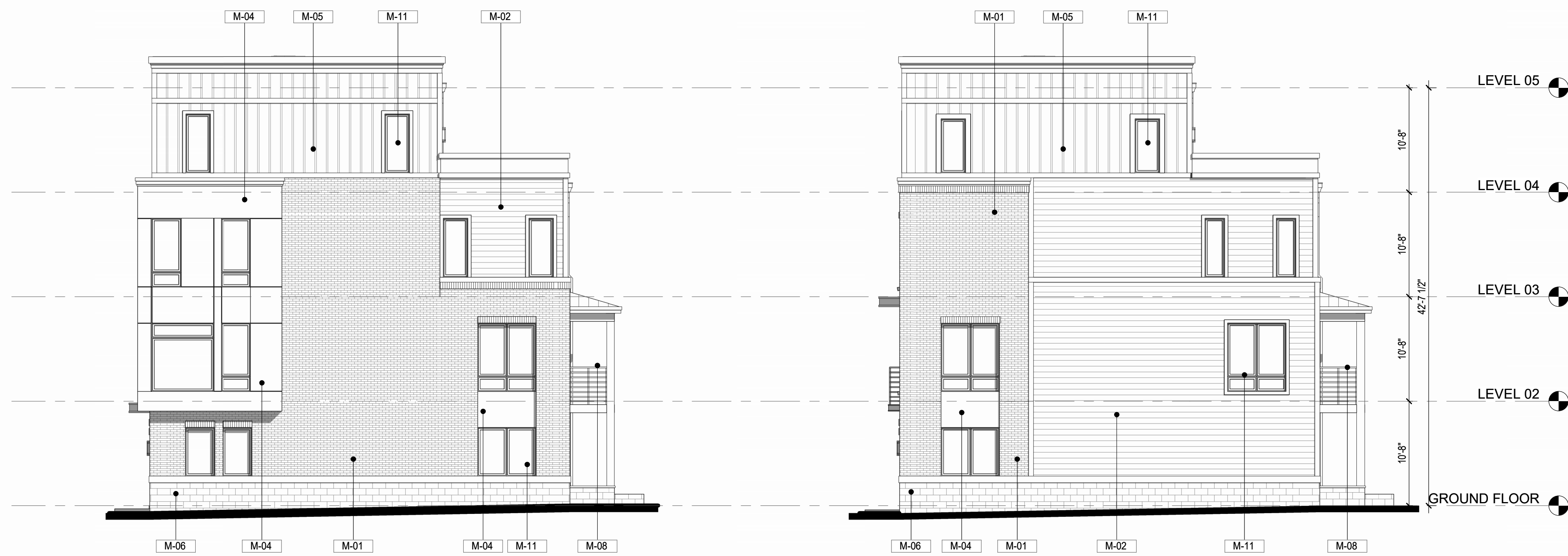
6 SIDE ELEVATION - HV A.S-123 1/8" = 1'-0" WALL OPENING:14% 5 SIDE ELEVATION - LV A.S-123 1/8" = 1'-0" WALL OPENING:9%
