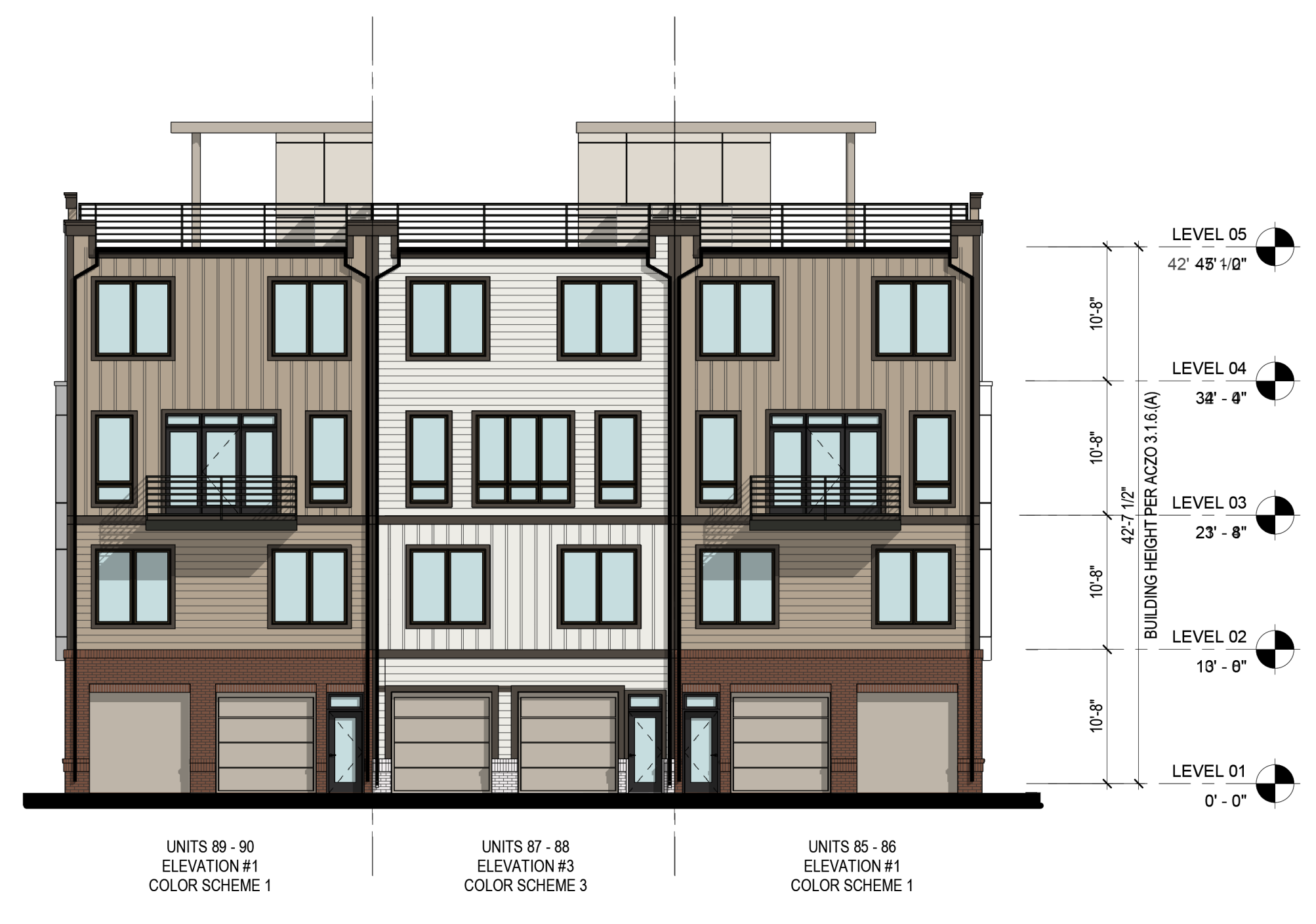
4 BUILDING SL - REAR ELEVATION A.SL-002 1" = 10'-0"
