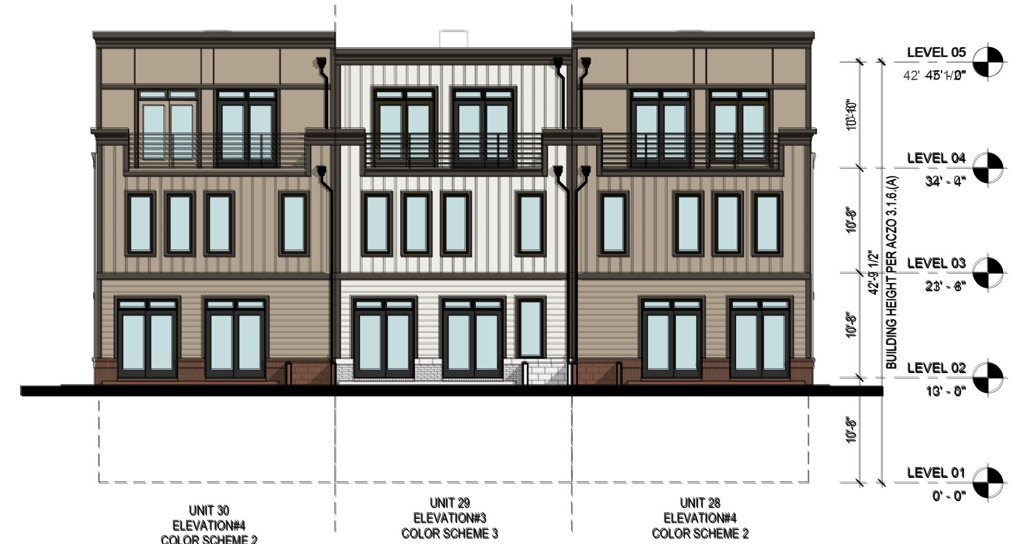
2 | BUILDING SD - REAR ELEVATION A.SD-002 1" = 10'-0"
