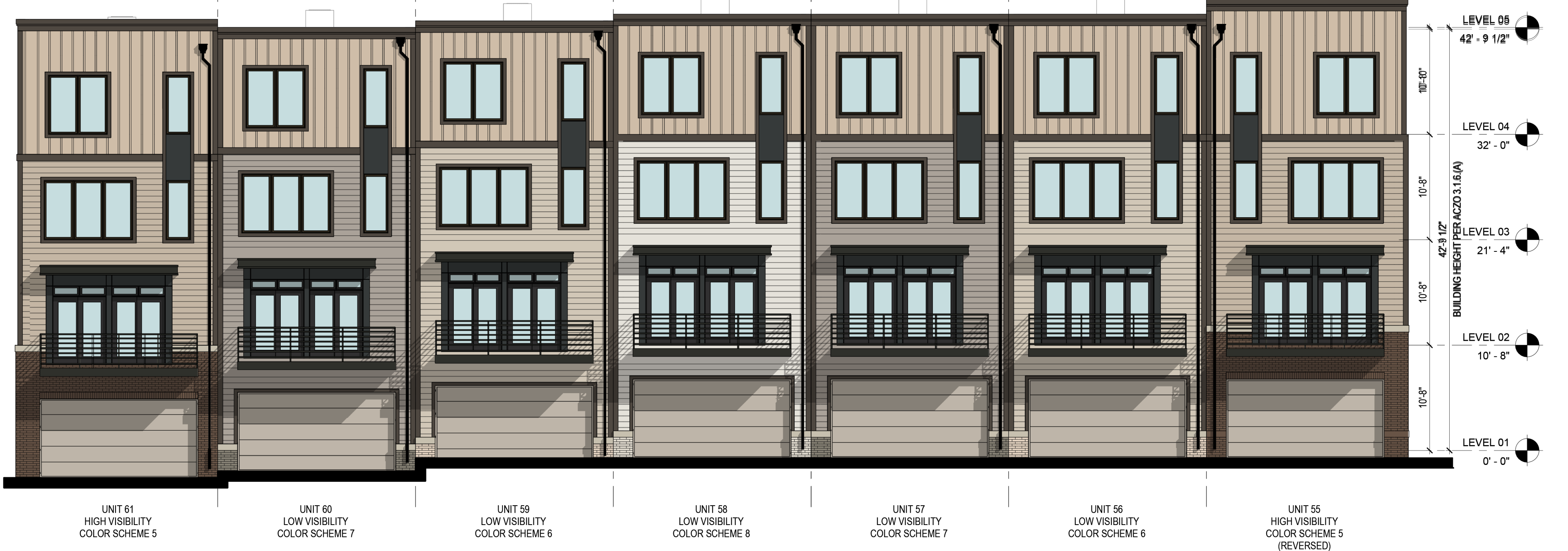
2 BUILDING SH - REAR ELEVATION A.SH-003 1/8" = 1'-0"
