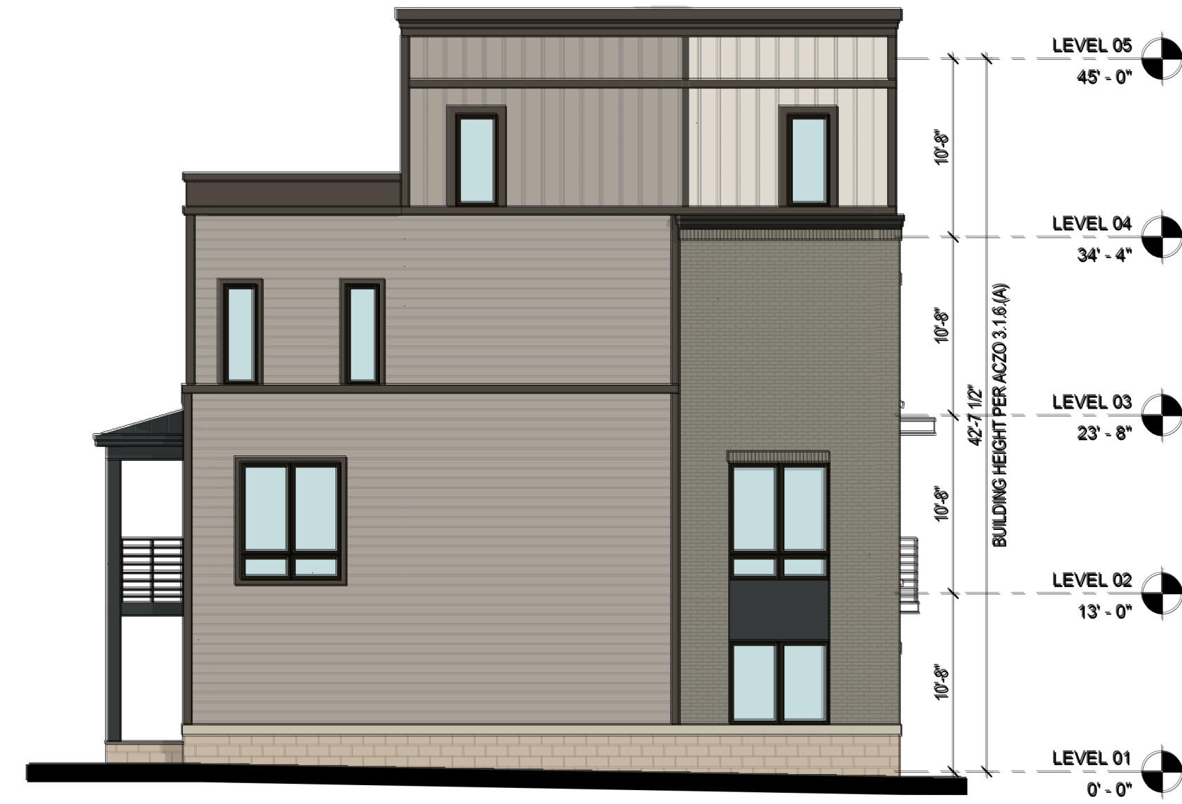
1 BUILDING SB - LEFT ELEVATION A.SB-004 1/8" = 1'-0"
