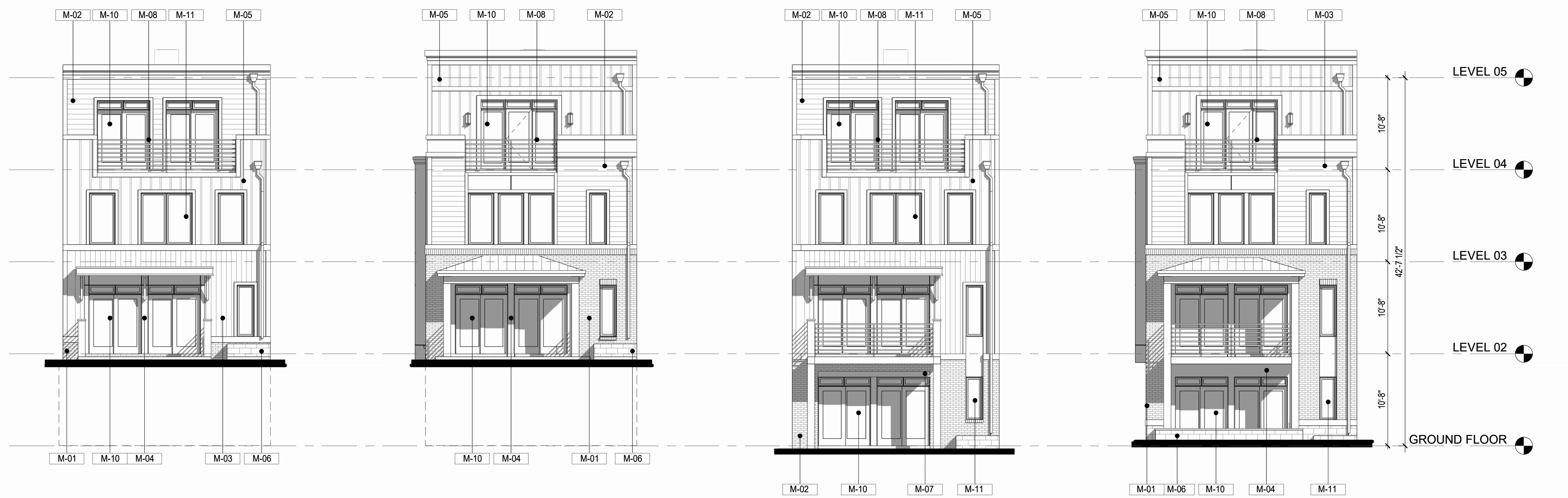
4 REAR ELEV. - INT - BURRIED A.S-123 1/8" = 1'-0" WALL OPENING:26% 3 REAR ELE. - END - BURRIED A.S-123 1/8" = 1'-0" WALL OPENING:22% 2 REAR ELEV. - INT A.S-123 1/8" = 1'-0" WALL OPENING:36% 1 REAR ELE. - END A.S-123 1/8" = 1'-0" WALL OPENING:31%
