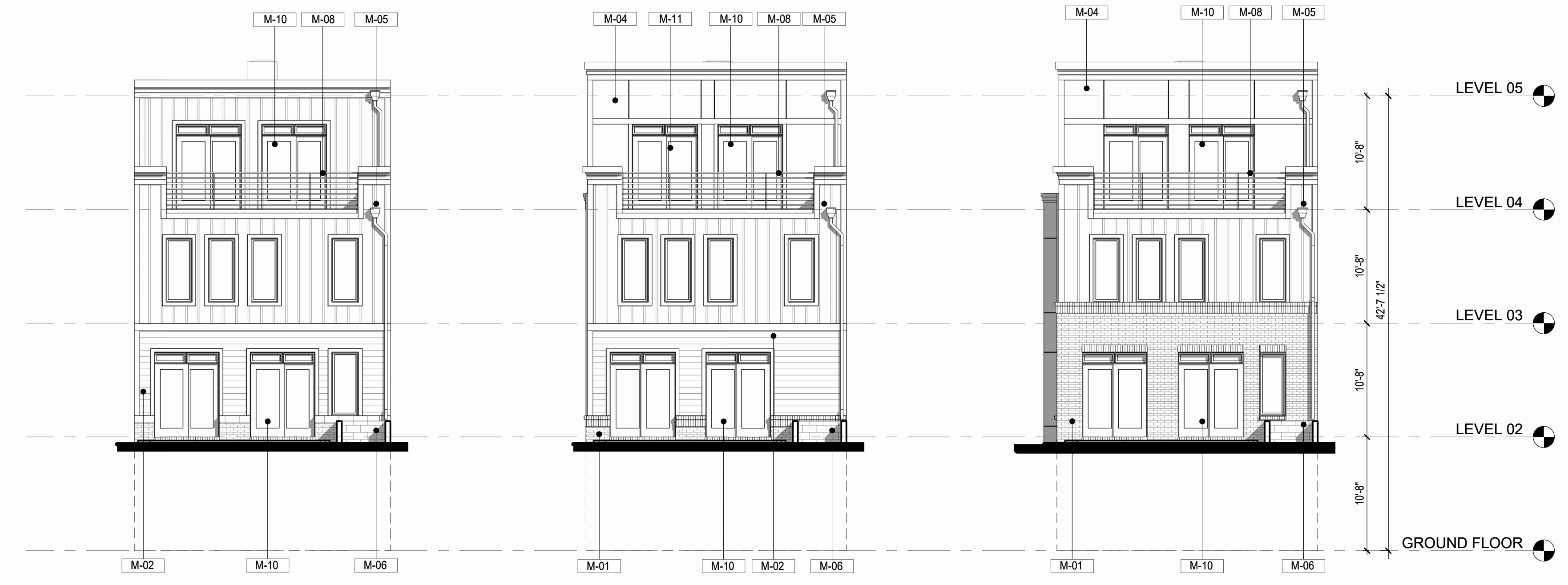
3 REAR ELEVATION #INT. A.S-133 1/8" = 1'-0" WALL OPENING:26% 2 REAR ELEVATION #4 END A.S-133 1/8" = 1'-0" WALL OPENING:23% 1 REAR ELEVATION #1 END A.S-133 1/8" = 1'-0" WALL OPENING:24%
