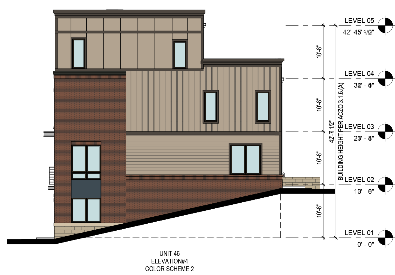
4 BUILDING SF - RIGHT ELEVATION A.SF-003 1" = 10'-0"
