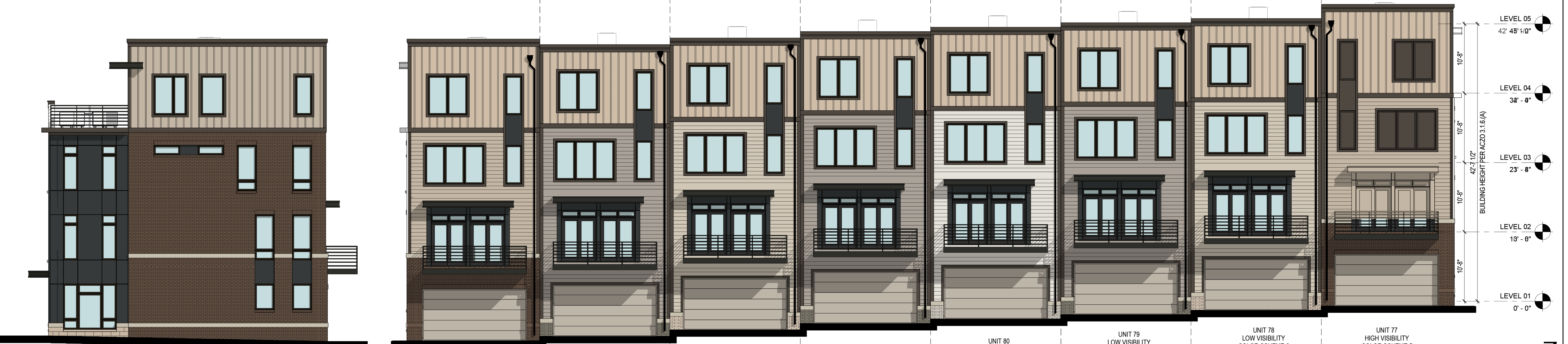
2 BUILDING SK - REAR ELEVATION A.SK-003 1/8" = 1'-0" UNIT 84 HIGH VISIBILITY COLOR SCHEME 5 UNIT 83 LOW VISIBILITY COLOR SCHEME 7 UNIT 82 LOW VISIBILITY COLOR SCHEME 6 UNIT 81 LOW VISIBILITY COLOR SCHEME 7 UNIT 80 LOW VISIBILITY COLOR SCHEME 8 UNIT 79 LOW VISIBILITY COLOR SCHEME 7 UNIT 78 LOW VISIBILITY COLOR SCHEME 6 UNIT 77 HIGH VISIBILITY COLOR SCHEME 5
