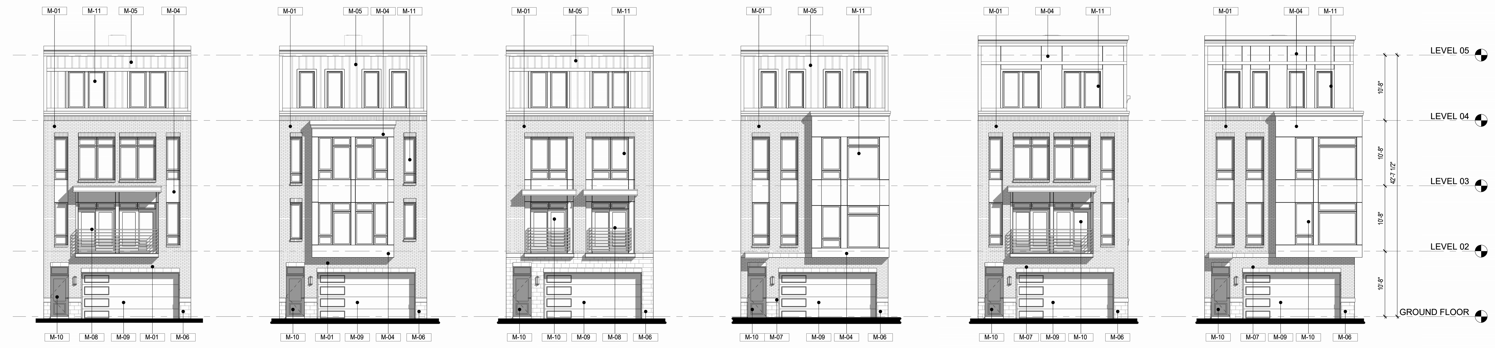
6 FRONT - ELEV. #4 INT WALL OPENING:43% 5 FRONT - ELEV. #3 INT WALL OPENING:38% 3 FRONT - ELEV. #2 INT WALL OPENING:37% 4 FRONT - ELEV. #1 INT WALL OPENING:37% 2 FRONT - ELEV. #4 END WALL OPENING:41% 1 FRONT - ELEV. #1 END WALL OPENING:36%
