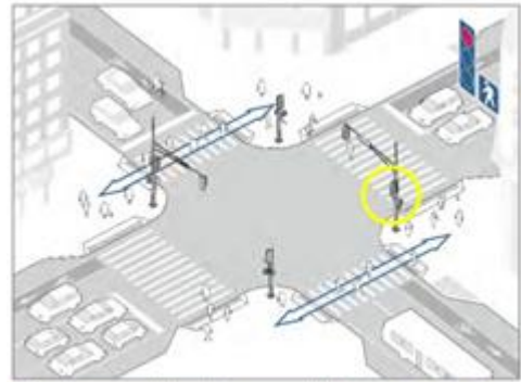
LPIs allow crosswalk flow before a green light is given for general travel lanes.
