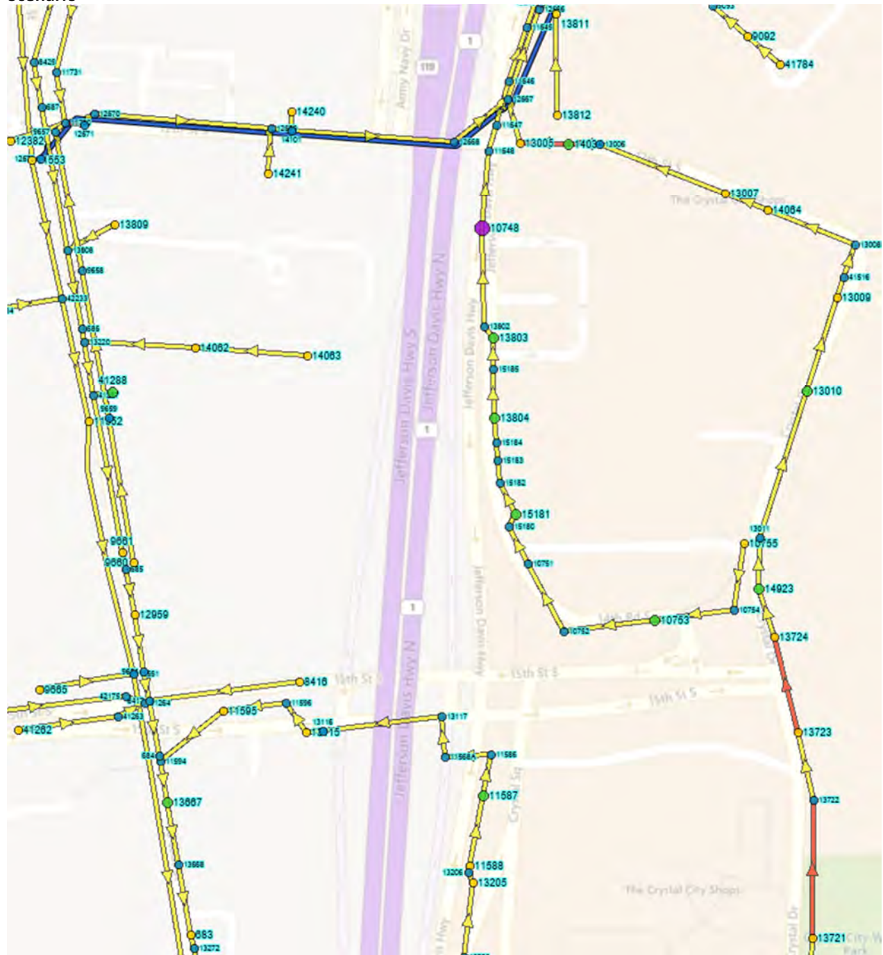
Figure 3-10. >90% Full-Flow Sewer Segments Along Crystal Drive in National Landing, Future 4X Planning Scenario
