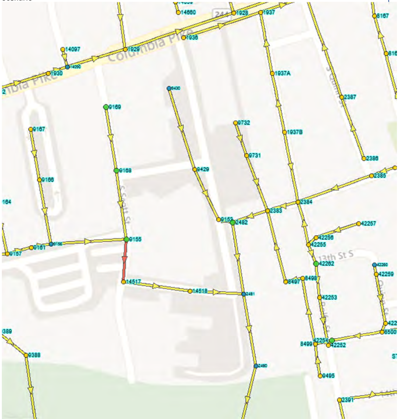
Figure 3-15. >90% Full-Flow Sewer Segment Along S. Scott St in Columbia Heights, Future 4X Planning Scenario
