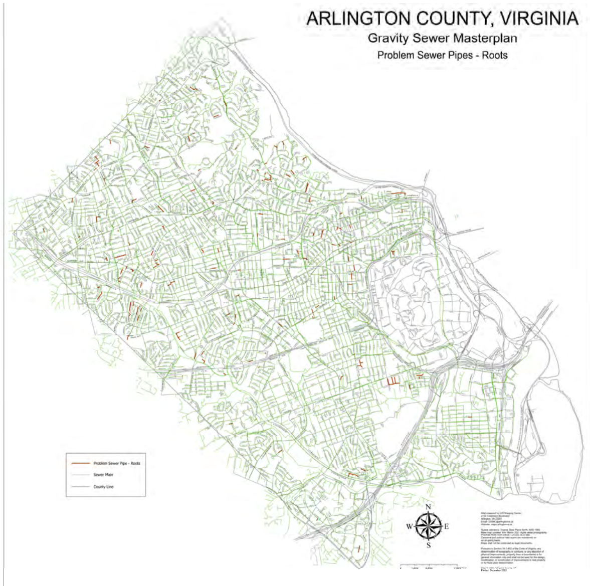
Figure 2-7 Sewer Segments Regularly Treated to Control Roots
