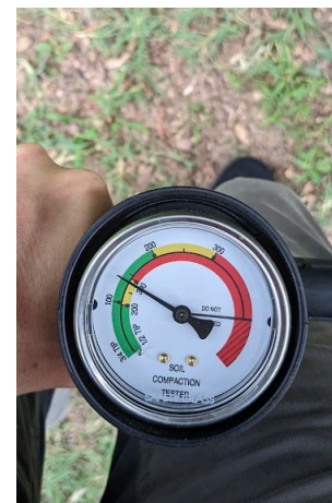
Figure 1: Using a soil penetrometer
