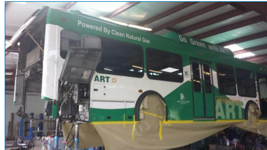
ART bus undergoing rehab work
