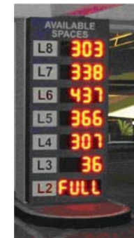
Display board for an electronic parking space count system.
