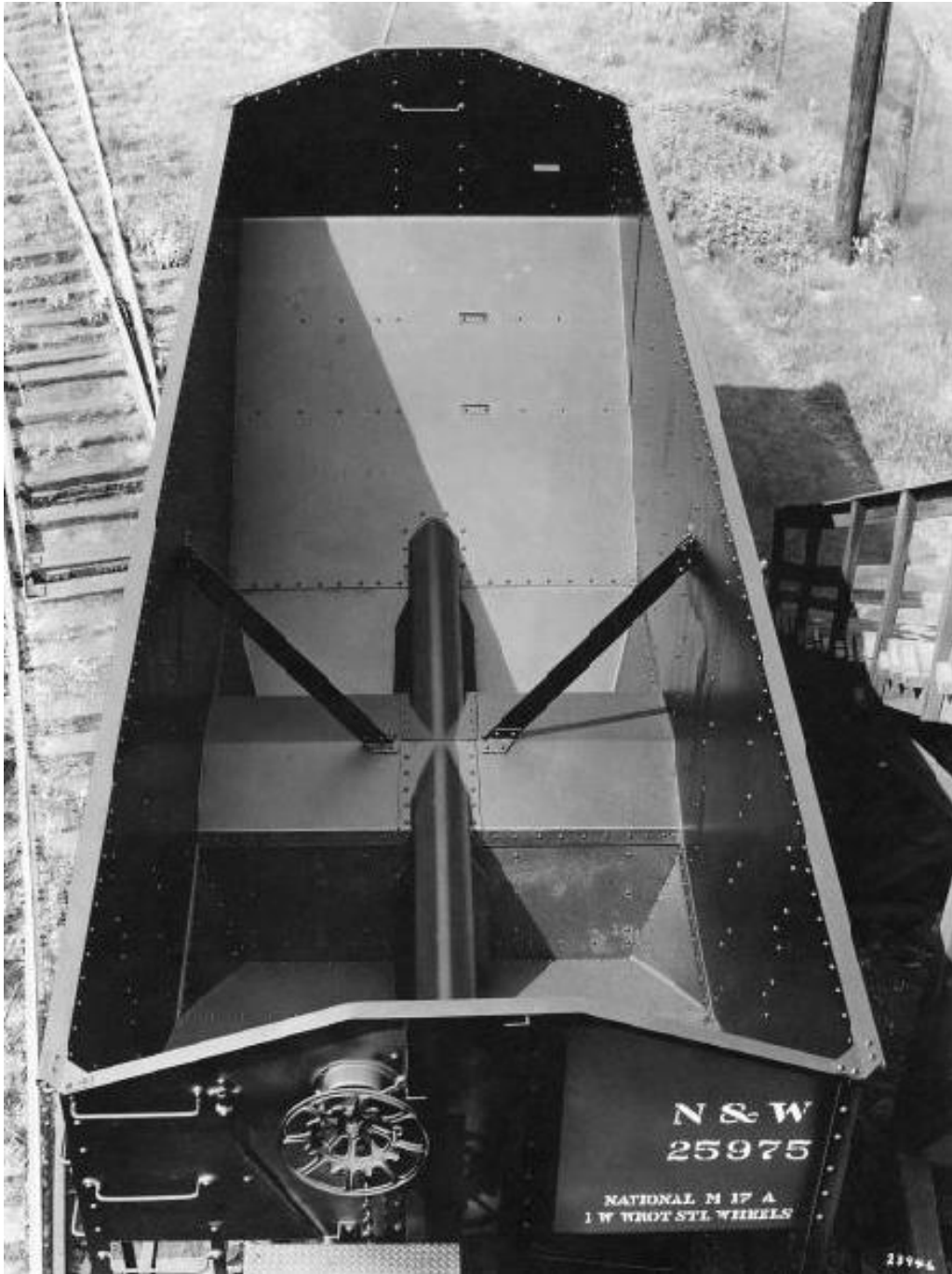
Figure 2: Interior of a hopper car. The bottom doors opened to release the coal. Source: Virginia Tech, "Virginia Tech ImageBase," http://www.imagebase.lib.vt.edu .
