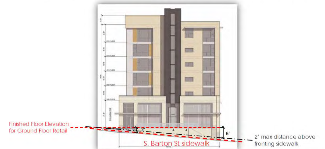
Exhibit 9a: Proposed modification for height of finished floor elevation on S. Barton Street
